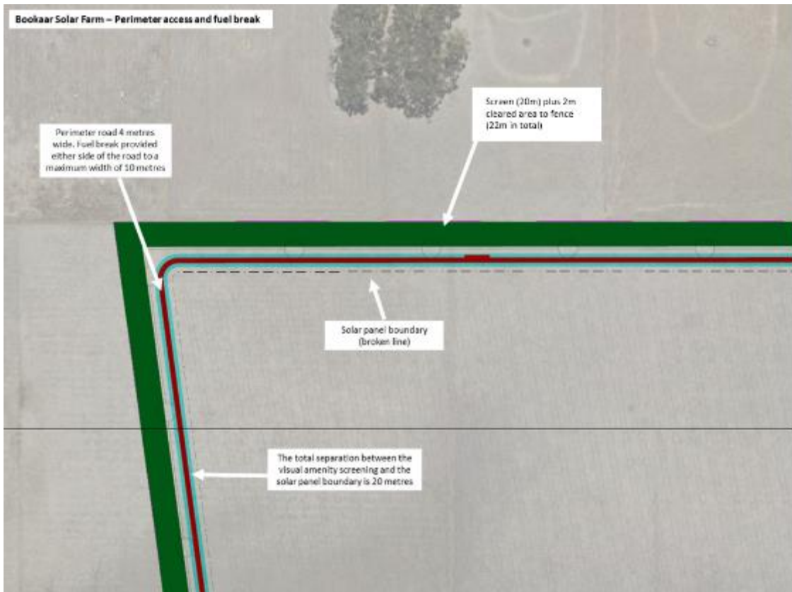
Figure 16 - Overview of management of bushfire risk along the north west Site boundary
