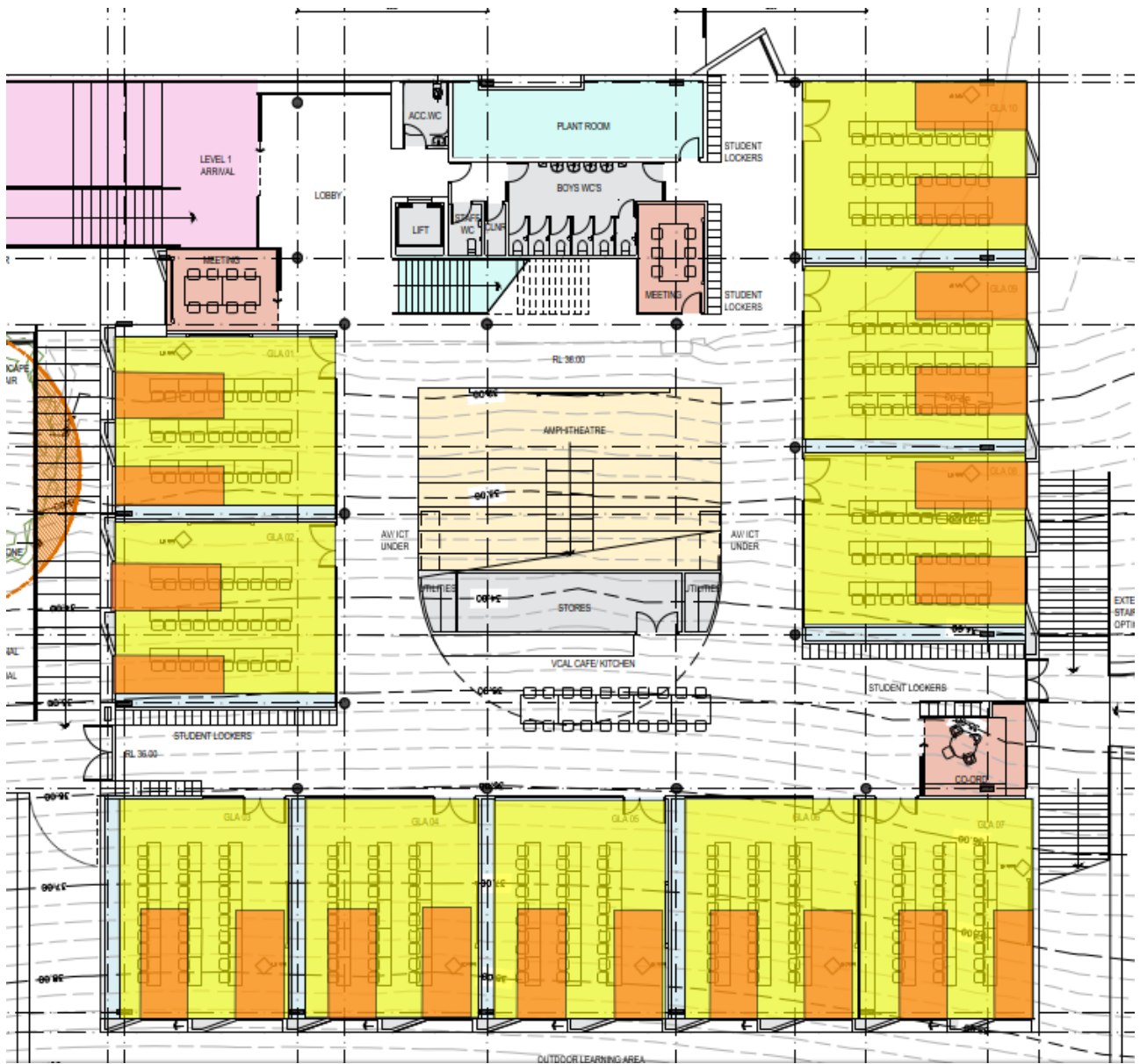
Figure 11: Daylight zone of compliance of all the level 1 classrooms of the development.
