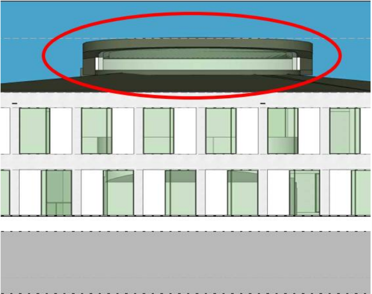
Figure 13: Three-sided windows that provide light to the Atrium Amphitheatre on the Level 2 of the development.
