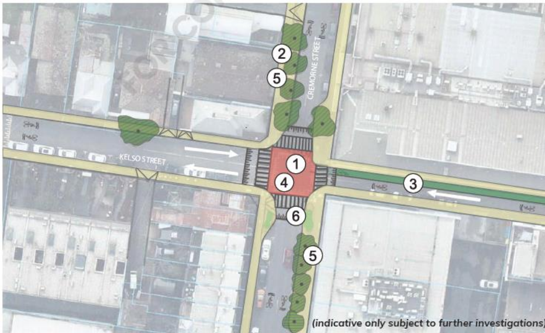
Figure 12: Cremorne Street and Kelso Street medium-term intersection concept design. Kelso Street future layout will be one-way westward, and Cremorne Street is one way south with a two way bike lane (Source: Revised Cremorne Urban Design Framework 2023)
