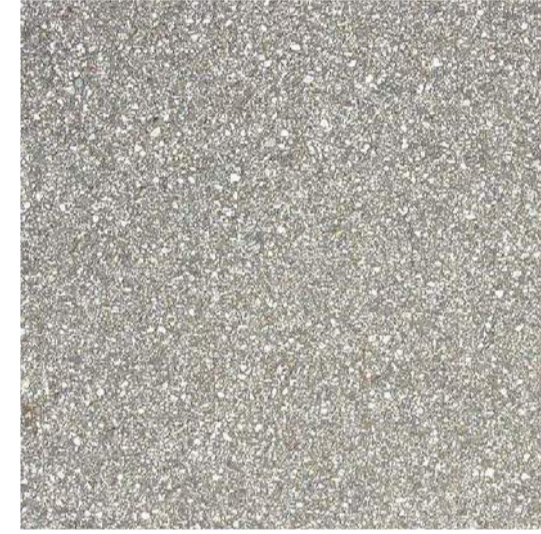
FPV-01: EXTERNAL PAVING EXPOSED AGGREGATE PAVING
