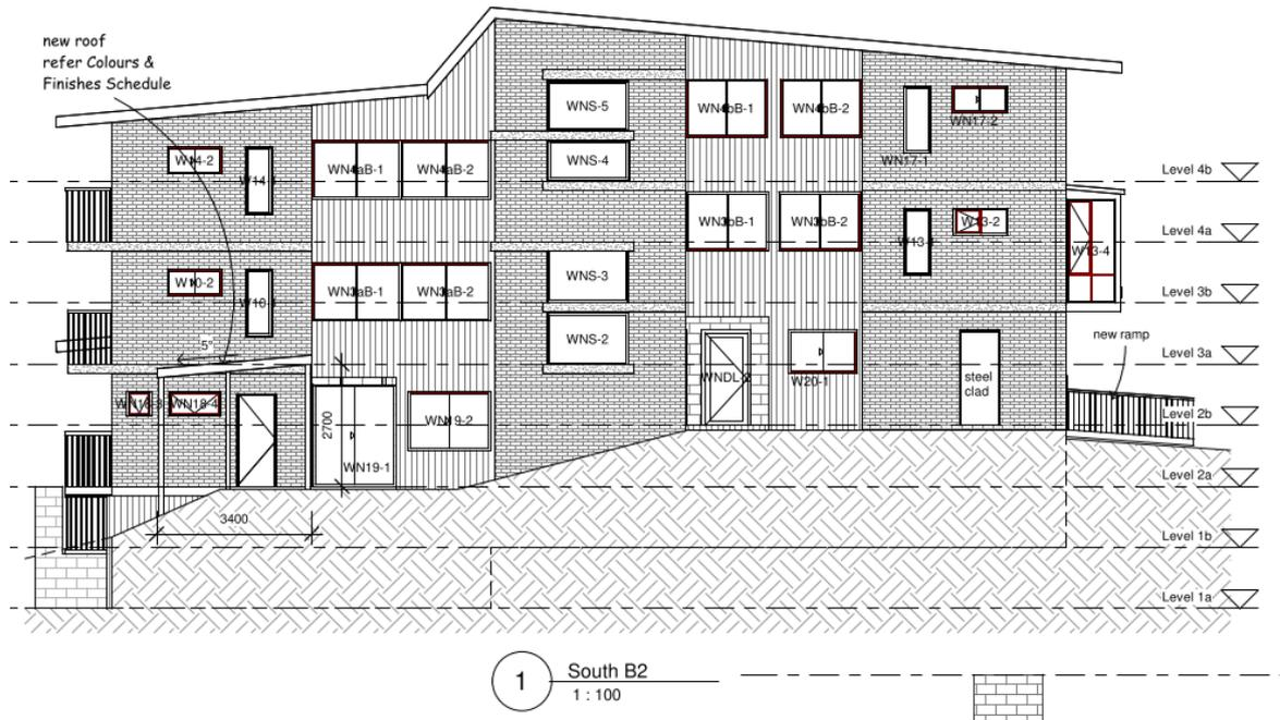
Figure 9 Proposed southern elevation Building 2, including entrance pergola to Unit 18
