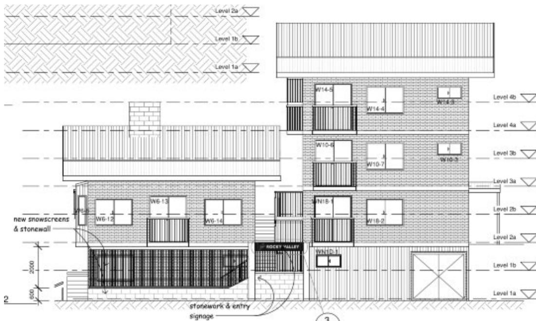
Figure 5 Proposed west elevation, including stone wall/ columns, snow screens and signage
