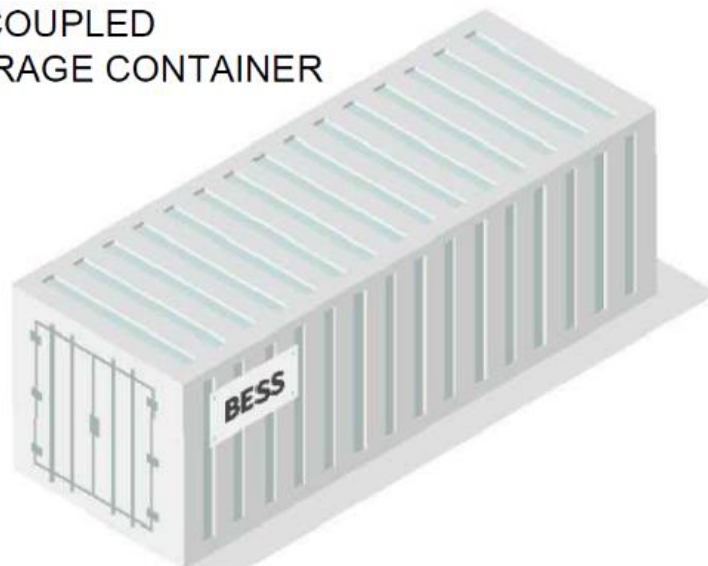
Figure 6. DC-Coupled Energy Storage Container (dimensions of 13m x 3m x 2.5m)
