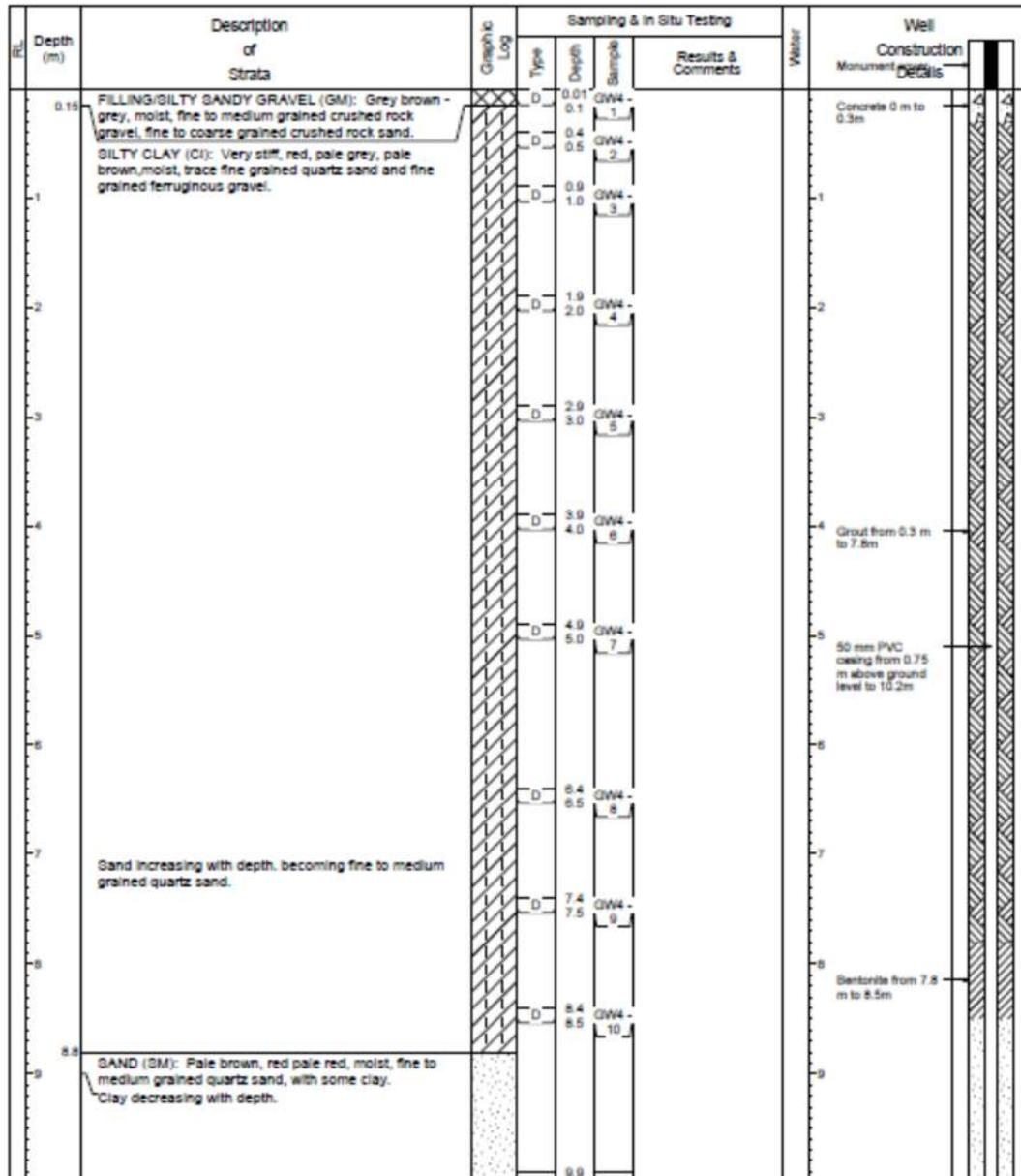
RIG: DB500 DRILLER: Aqua Drilling & Grouting LOGGED: CJC CASING: 50 mm PVC
