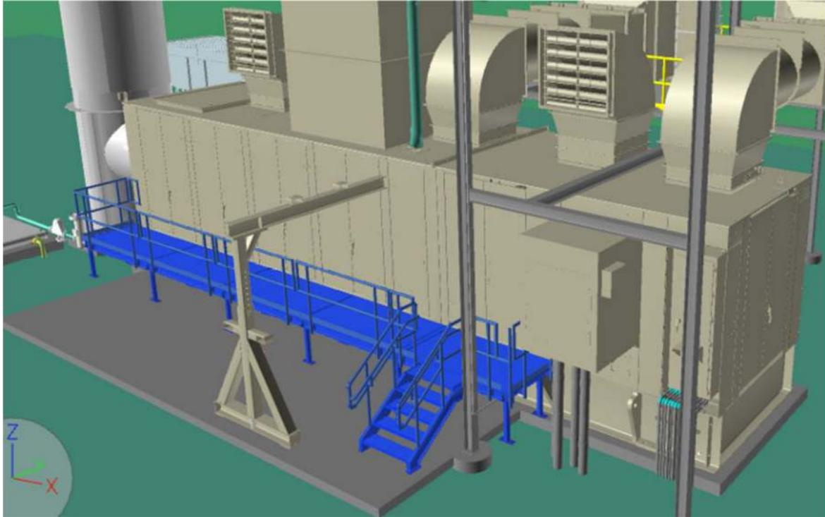
Figure 4: Preliminary 3D model of Titan 130 gas turbine generator, including air inlet filter & enclosure vent filter, access platforms and support structures
