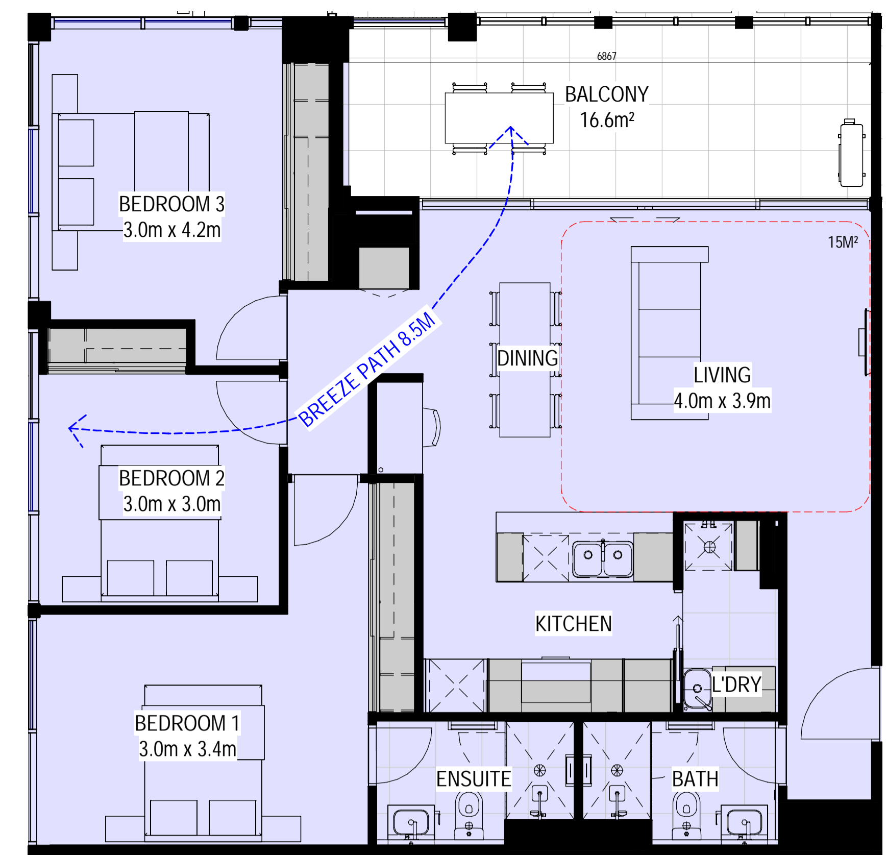
TYPE P 3 BEDROOM APARTMENT INTERNAL AREA - 105.1M 2 BALCONY - 16.7M 2 2 INSTANCES INTERNAL STORAGE - 18.8M 3 OVERALL STORAGE - 23.7M 3
