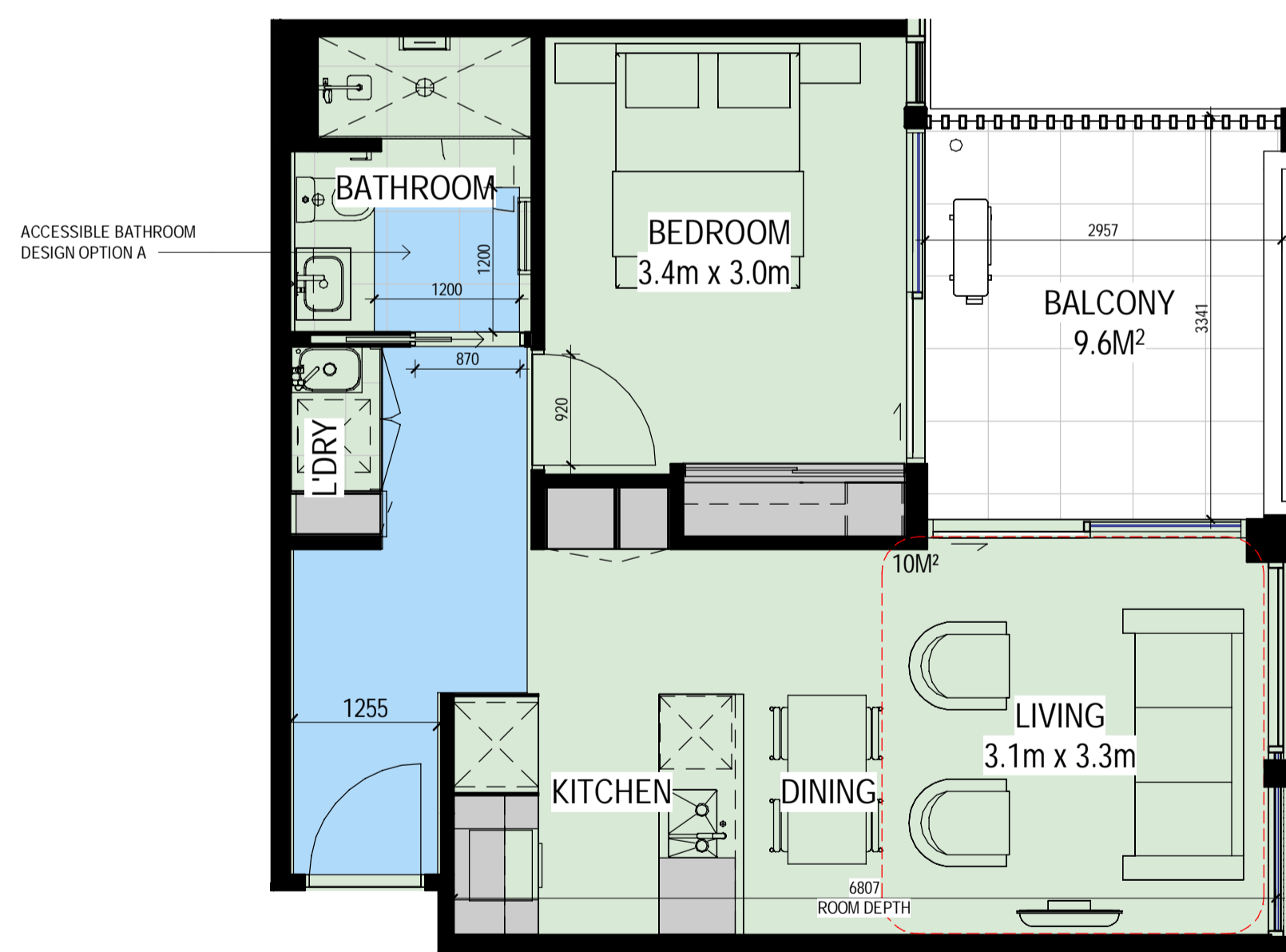
TYPE E 1 BEDROOM APARTMENT INTERNAL AREA - 52.1M 2 BALCONY - 9.6M 2 22 INSTANCES INTERNAL STORAGE - 6.4M 3 OVERALL STORAGE - 11.3M 3
