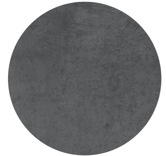
Precast Concrete 'dark grey' pigmented concrete to the green breaks to help accentuate and break down building mass.
