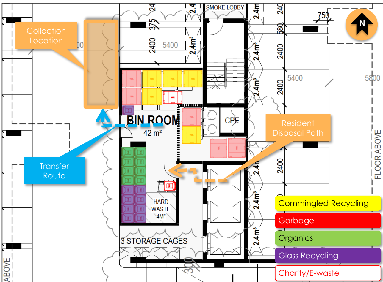
Figure 3 Bin Storage Room – Residential (Basement)
