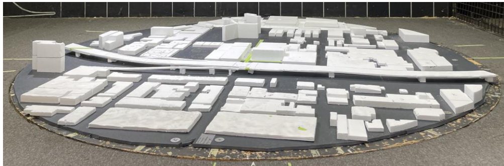
Figure 21: Overall view of the proposed development model in the wind tunnel (existing).
