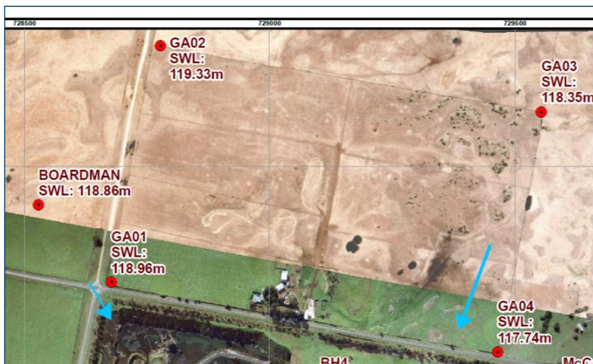
Figure 4: Groundwater monitoring wells in NDA
