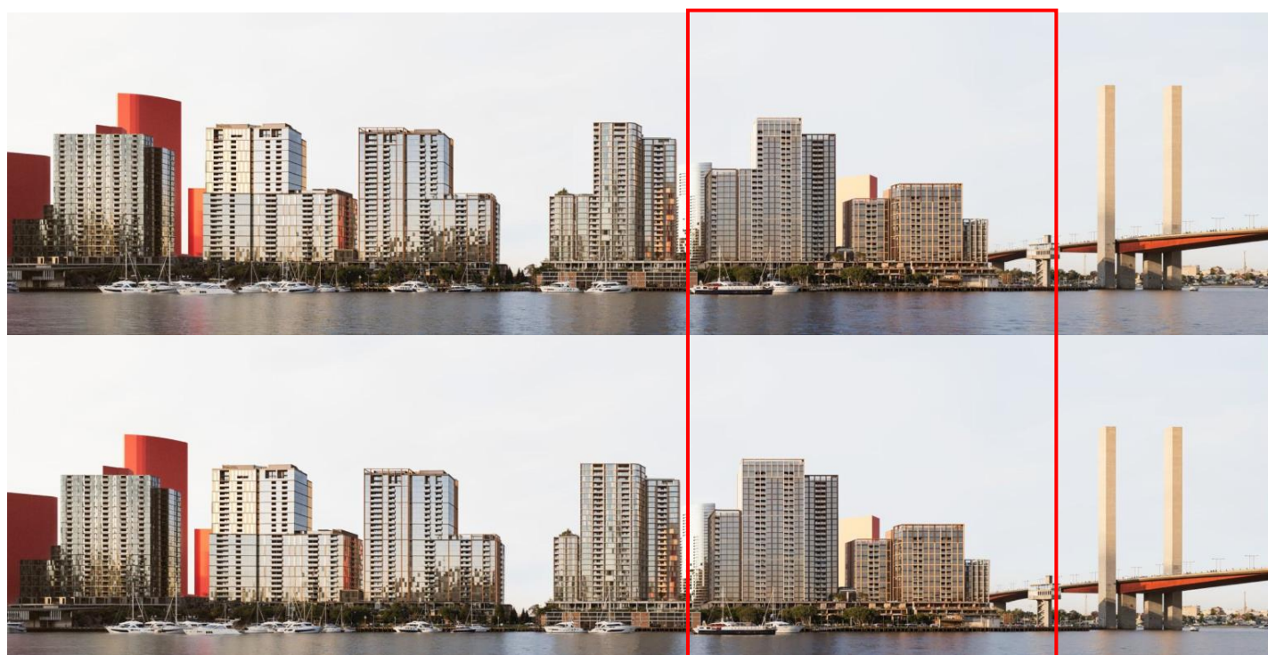
Figure 21: 50/50 mass split (top image) and 65/35 mass split (second image) when viewed in isolation from the north
