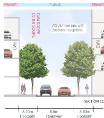
Figure 14: Dock Lane cross section
