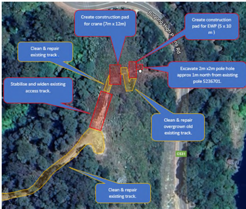
Figure 6 - MBTS-CLPS Pole Replacement 553 (BID 5236703) Detail
