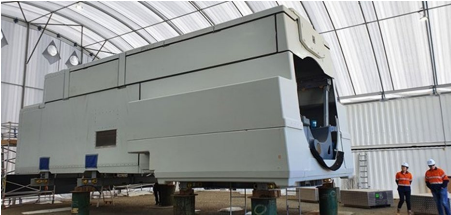
Photo 3.6 Example of a Nacelle for a 5.3 MW WTG at Bango Wind Farm
