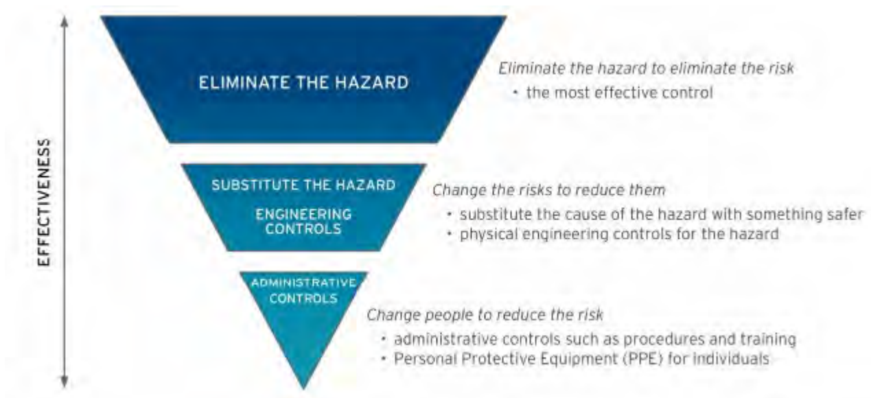
Figure 4-1 Hierarchy of controlling hazards and risks
