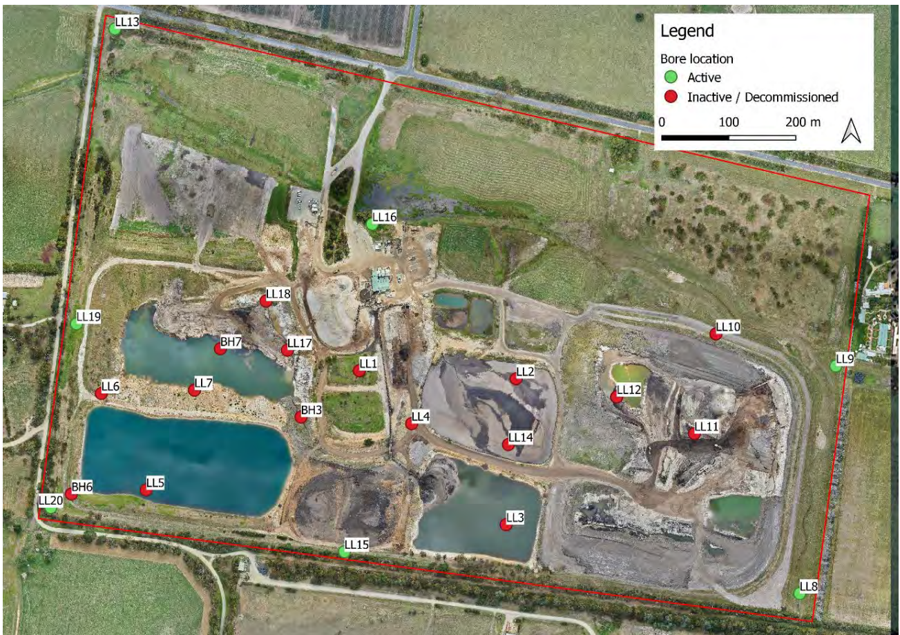
Figure 3-9 Site monitoring bores
