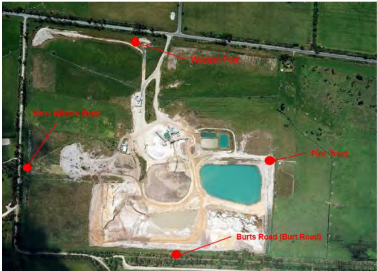
Figure 2: Existing Dust Gauge Locations (Source: Assessment of Potential Dust Impacts, GHD for Hanson Construction Materials, May 2013)
