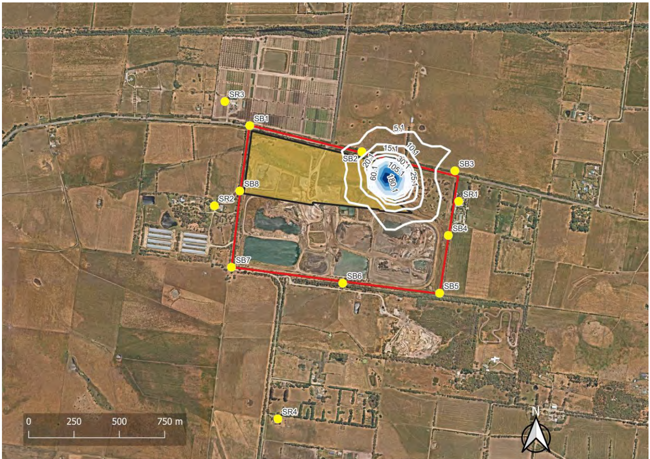
Figure 10: Contour plot of CO (1 hr average) showing compliance with all coordinates modelled in the grid
