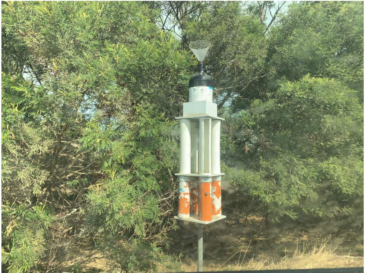
Figure 3: Dust Gauge (Burt Road)
