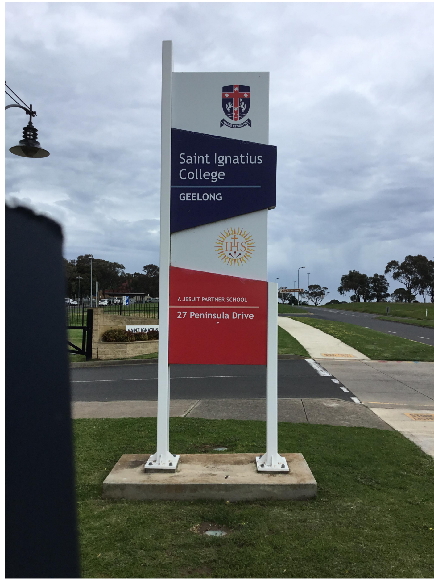
EXISTING FRONT SIGNAGE 1 - PENINSULA DRIVE DIMENSIONS: 3m(H) x 1m(W) HEIGHT ABOVE NGL: 1m ILLUMINATED: YES, 2 x GROUND LIGHTS HOURS: 7PM TO 6AM (DAILY) BAFFLES PROVIDED: NO
