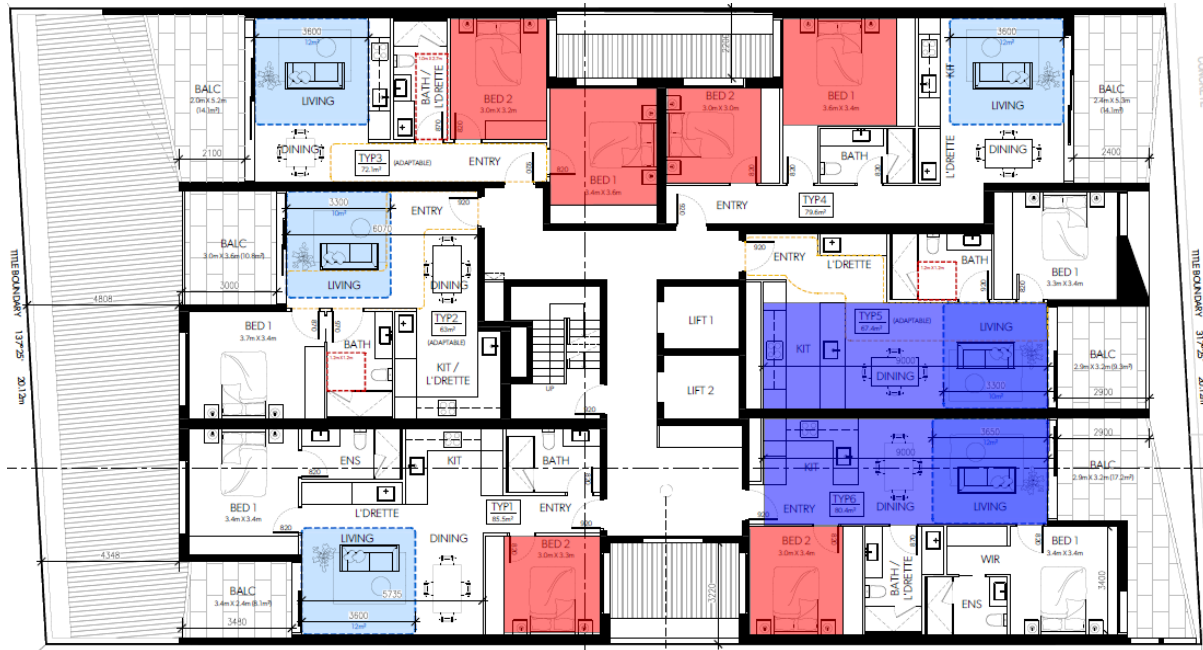
Figure 11: Markup of non-DTS rooms on Levels 4 to 11
