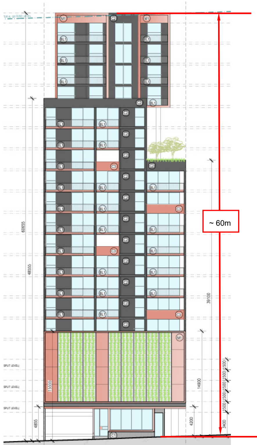
Figure 2: Northeastern elevation of the proposed development.
