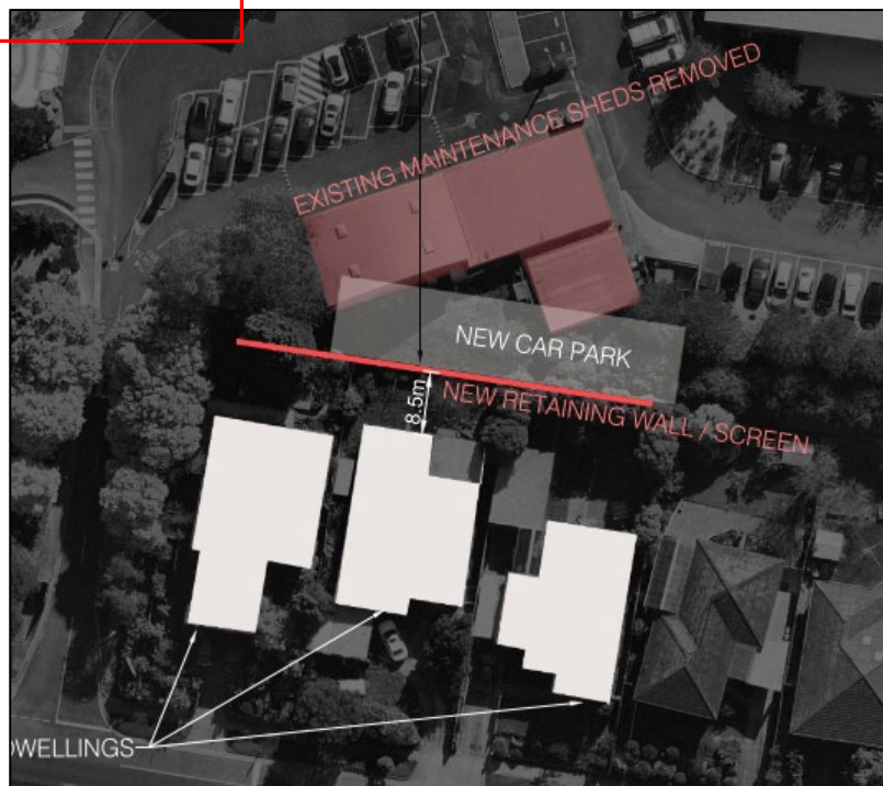
Figure 1: Excerpt from the landscape plan which shows the existing and proposed works as they relate to the southern boundary.
