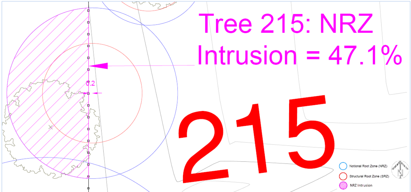
Figure 11 Tree 215 NRZ Intrusion
