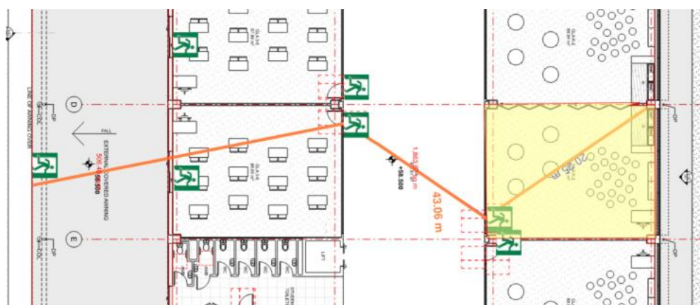
Figure 13: Ground Floor – GLA's with excessive travel to the nearest of two exits.
