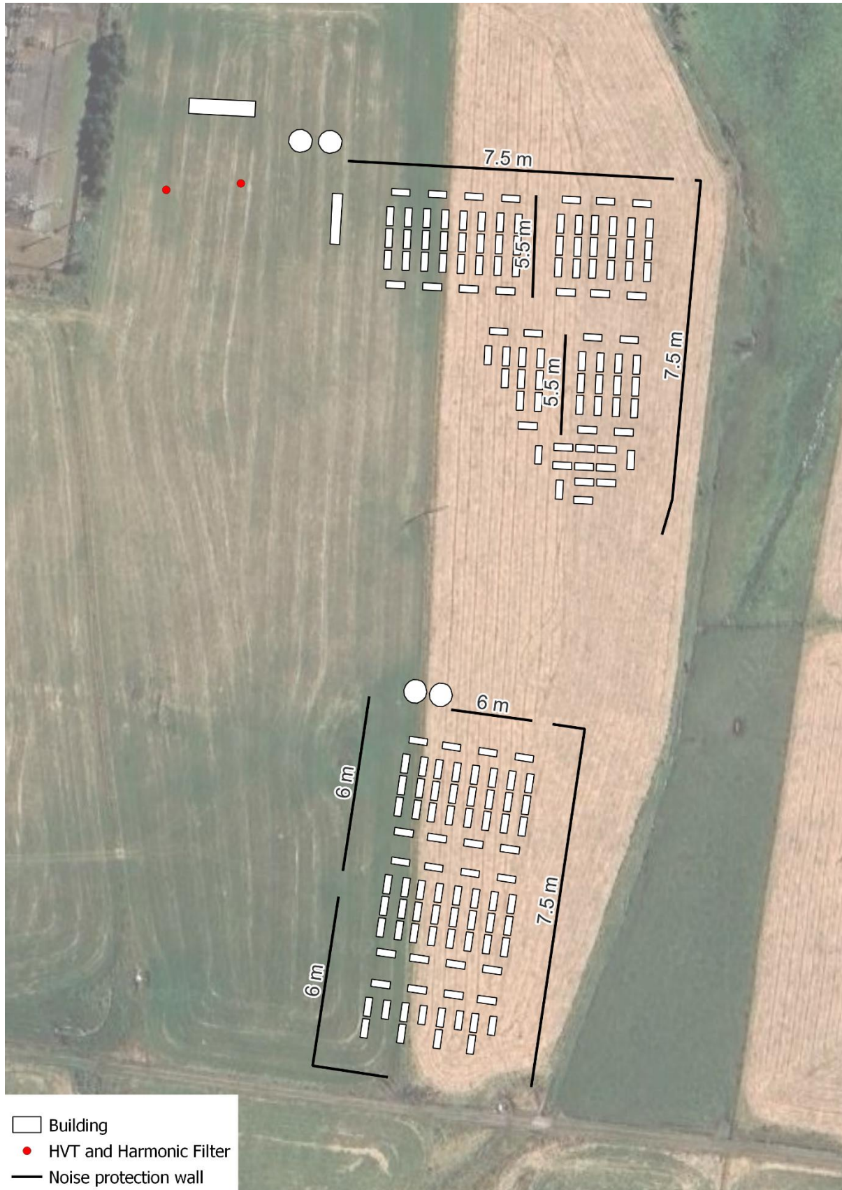
Figure 2 BESS Detail Showing Noise Wall Locations
