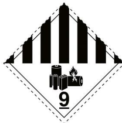
Figure 7: Placard for storages of Class 9 packaged dangerous goods
