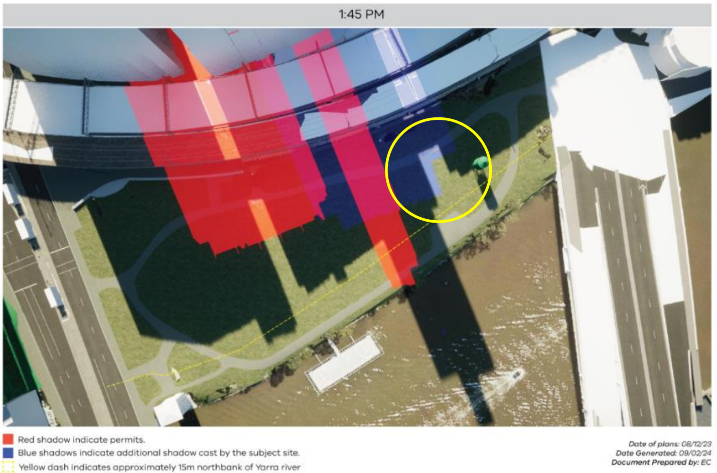
Figure 26 - Shadow analysis prepared by DTP's 3D visualisation team showing time where additional shadows occur (1:45pm on 22 June)
