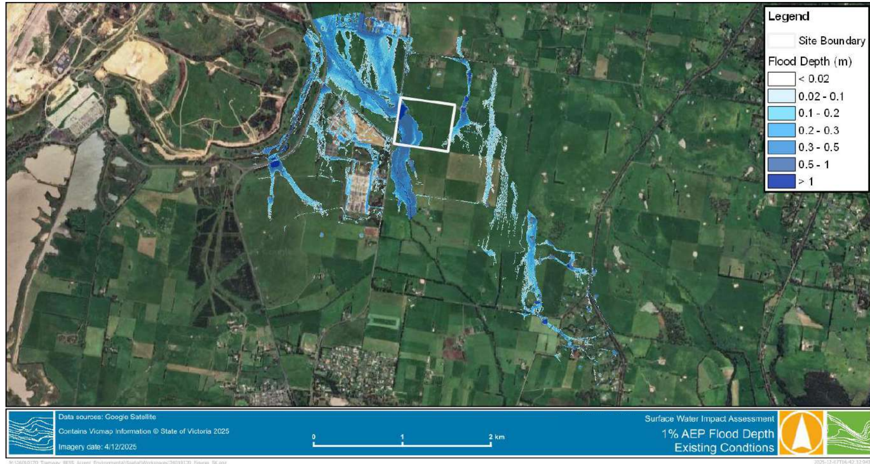
Figure 4-1 1% AEP Flood Depth – Existing Conditions
