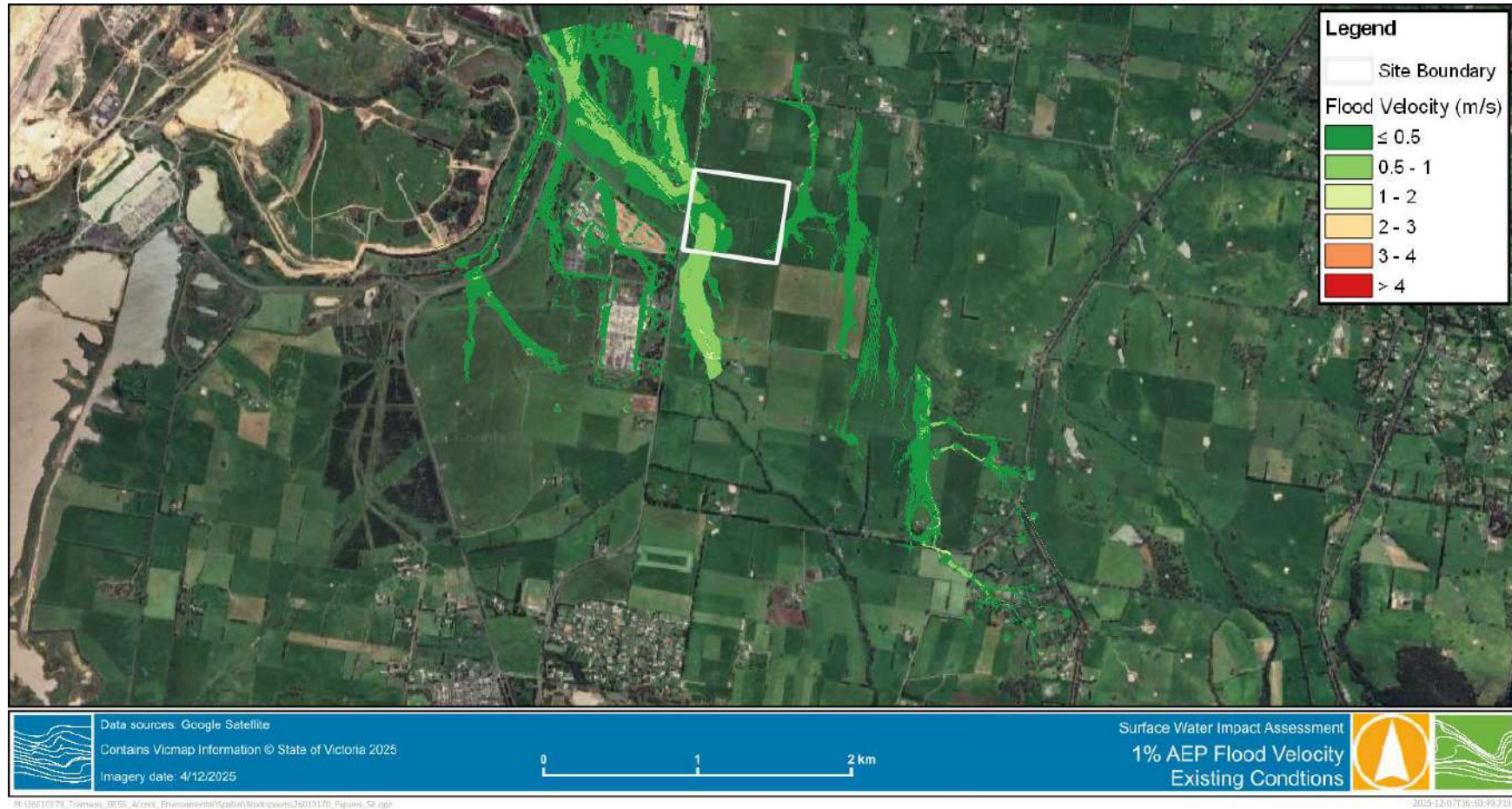
Figure 4-3 1% AEP Flood Velocity – Existing Conditions
