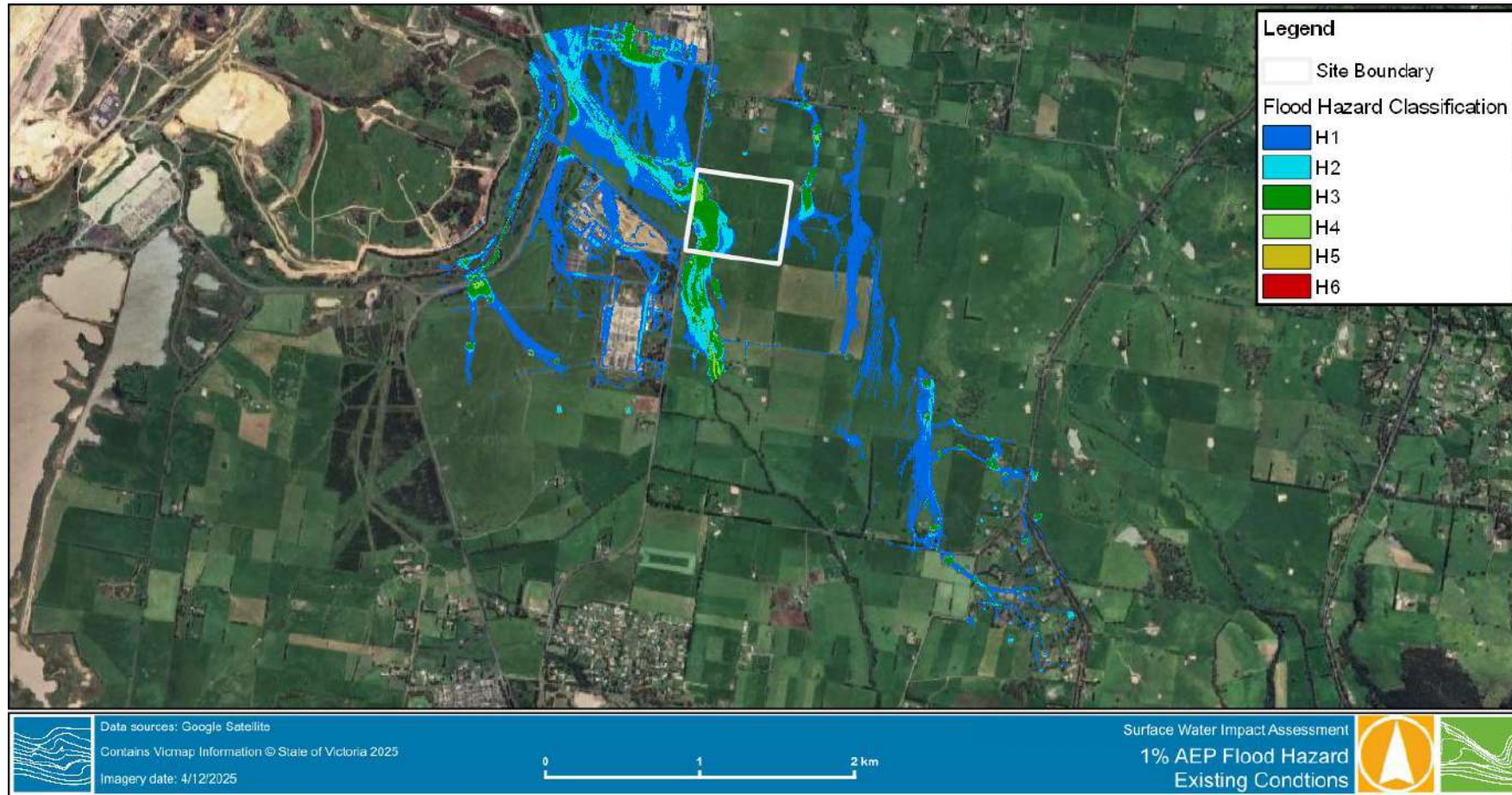
Figure 4-5 1% AEP Flood Hazard – Existing Conditions
