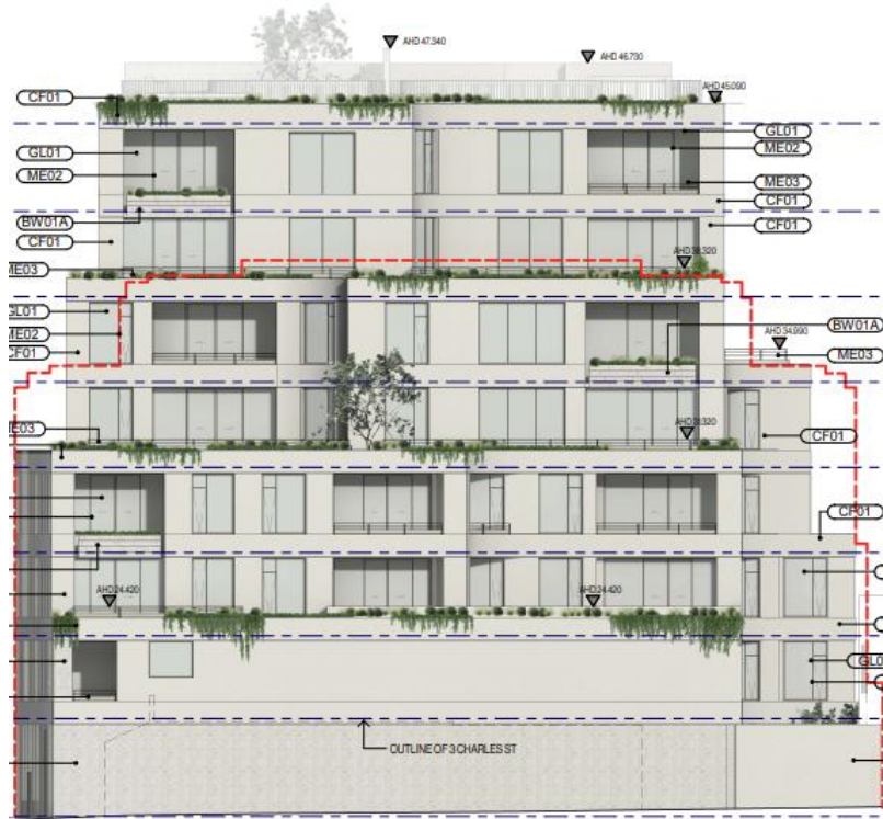
Figure 9: North elevation – red dotted line shows outline of existing permitted development (Source: Application)
