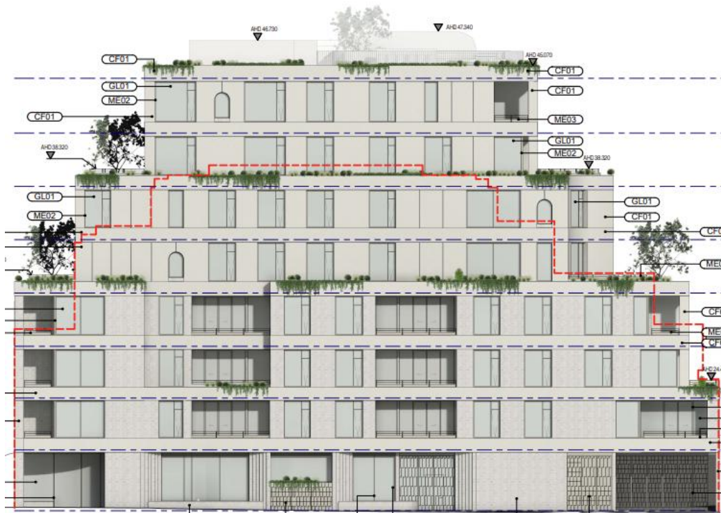
Figure 7: East elevation – red dotted line shows outline of existing permitted development (Source: Application)
