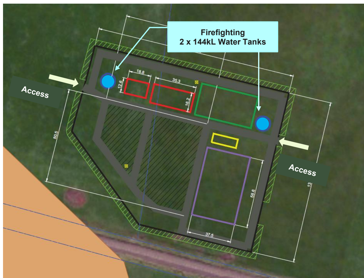
Figure 15 Location of Proposed Firefighting Water Tanks
