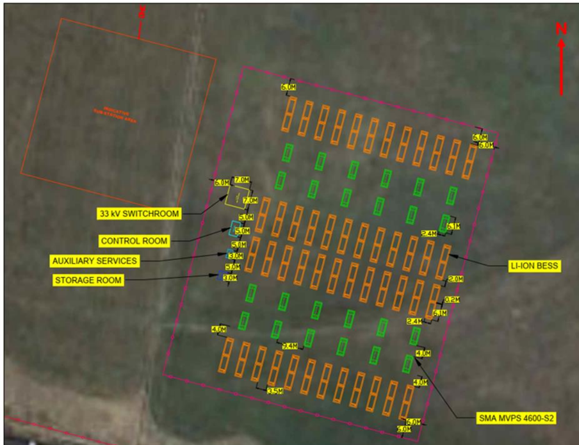
Figure 3 Proposed BESS development layout
