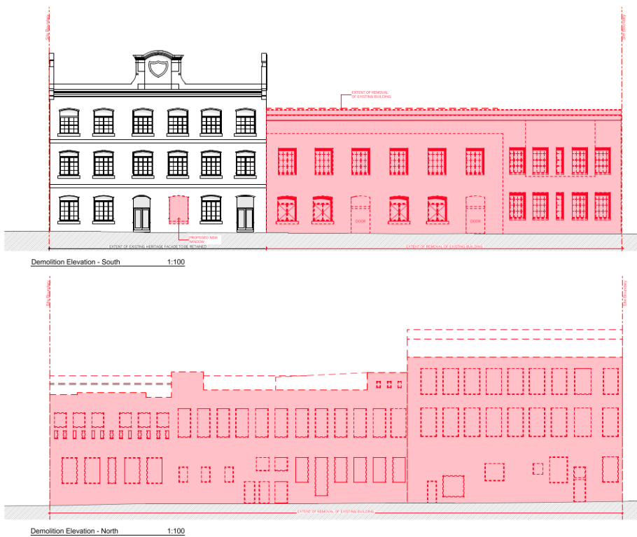
Figure 2 Proposed extent of demolition
