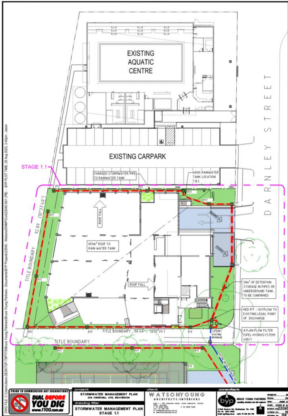
Figure 6 - Proposed Stormwater Concept Stage 1.1
