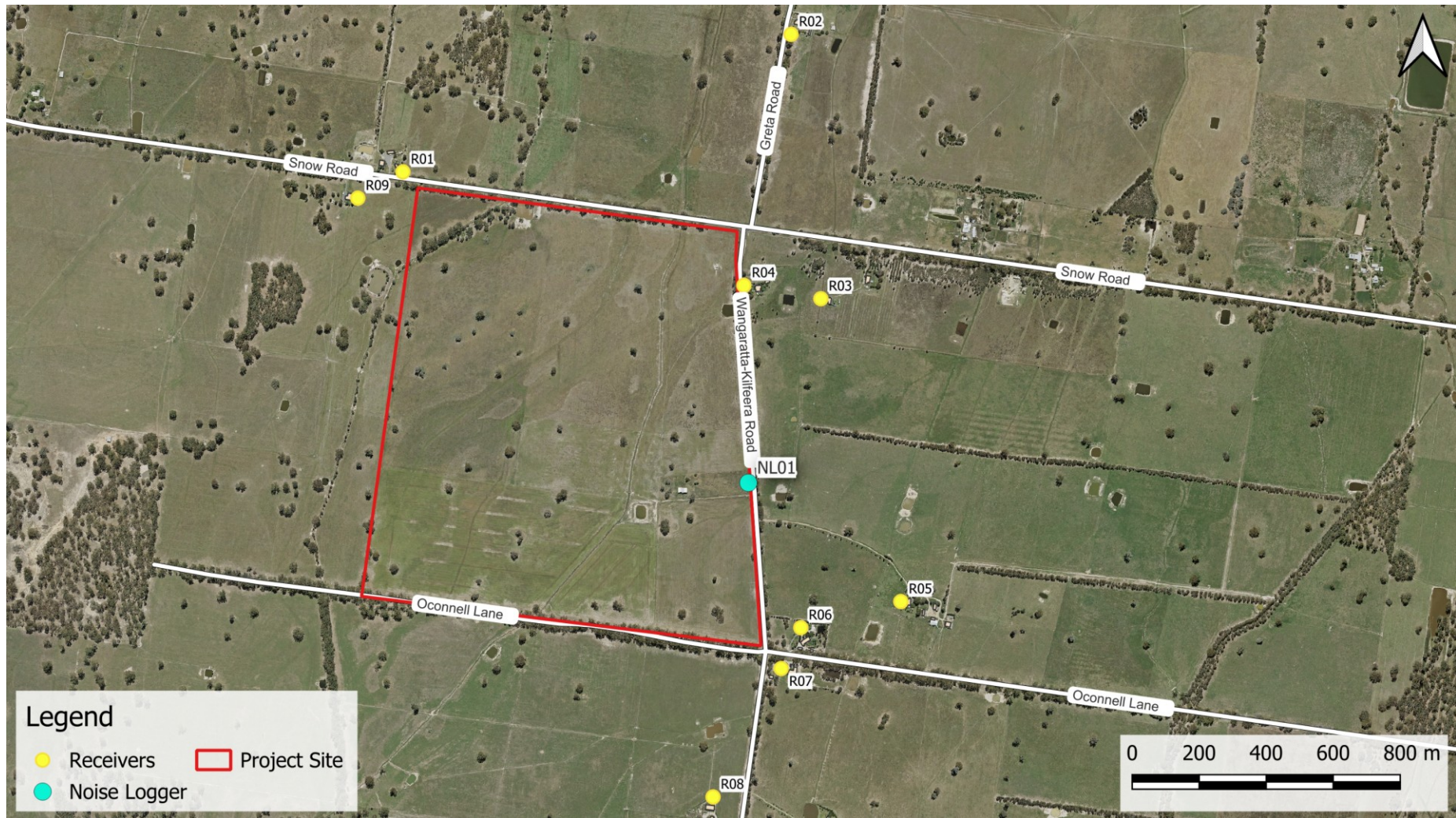
Figure 1 Site map, measurement locations and surrounding receivers – site map sourced from VicPlan
