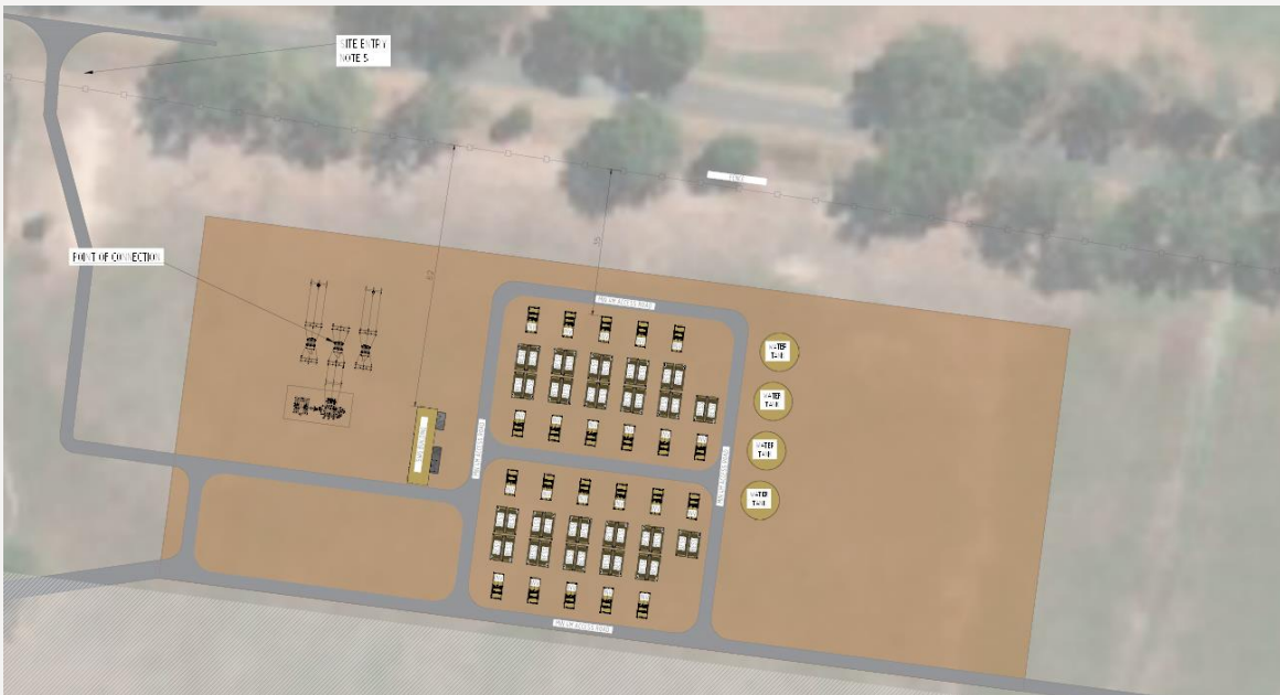
Figure 2 | Proposed BESS layout
