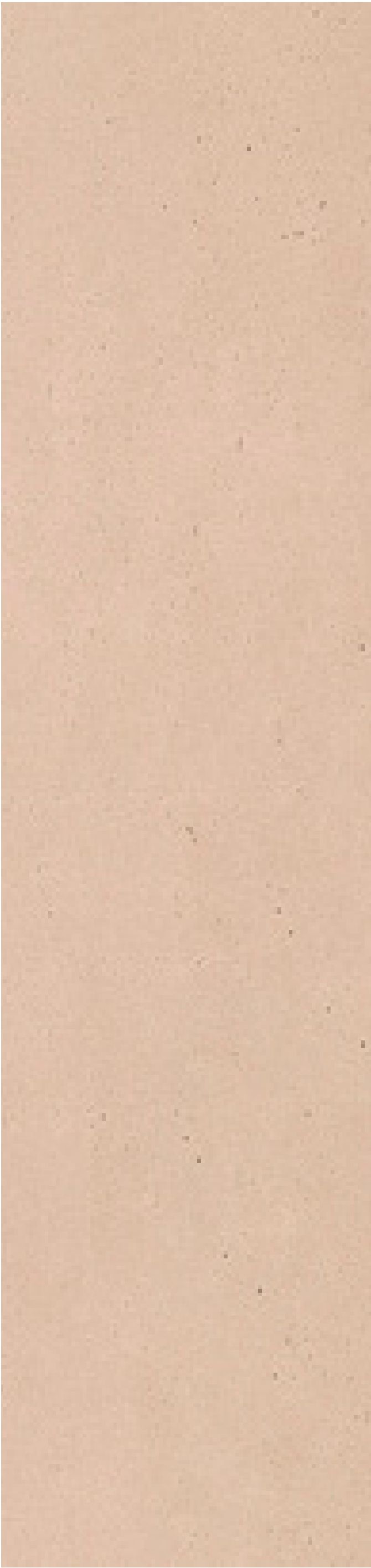
EF1 Light Pigment Concrete Finish. CCS 'Redbrick' oxide approx. 2bag/m3 based on site samples.
