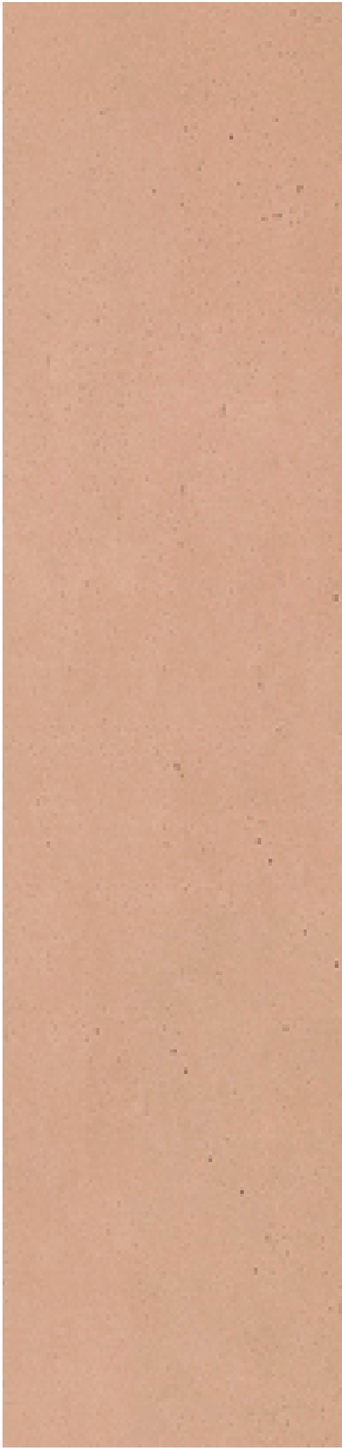
EF2 Dark Pigment Concrete Finish. CCS 'Redbrick' oxide approx. 3bag/m3 based on site samples.
