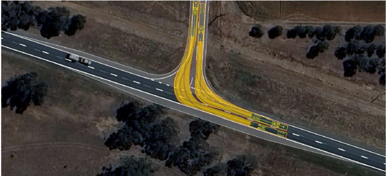
Figure 14: Right in / Left out turn path (Source: RMA Engineers, 2025).
