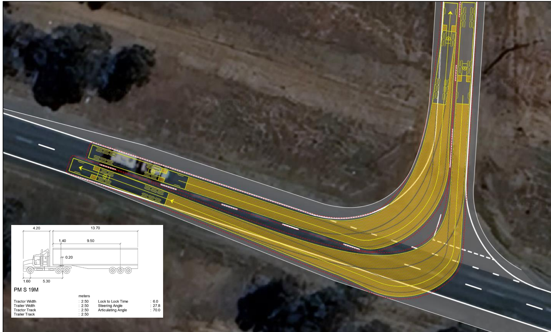
Murray Valley Highway / Heppell Road – 19m AV turn path – Left In / Right Out
