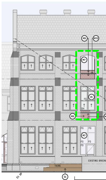
Figure 38: Extract of TP23 P2 1, showing alterations to the windows and walls on the first and second levels. Source: Y2 Architecture, 2023.
