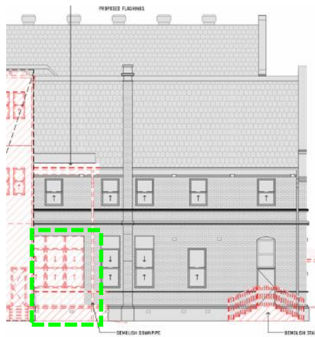
Figure 30: Extract of TP14 P2 E1, showing proposed demolition of windows and a section of wall at the North Wing's north façade (indicated in green). Source: Y2 Architecture, 2023.
