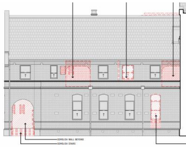
Figure 31: Extract of TP16 P2 E8, showing the proposed demolition of the North Wing at the south façade. Source: Y2 Architecture, 2023.
