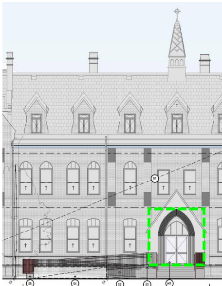
Figure 34: Extract of TP22 P2 1, showing the new double swing doors at the east façade of the original building. Source: Y2 Architecture, 2023.
