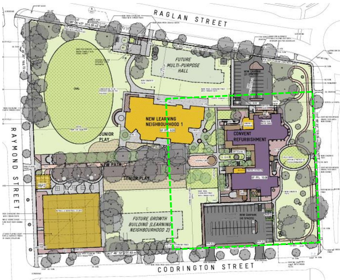
Figure 33: Extract of TP03 P2, proposed site plan. The HO curtilage is indicated in green, the Convent building in purple, and new buildings/additions in yellow. Source: Y2 Architecture, 2023.
