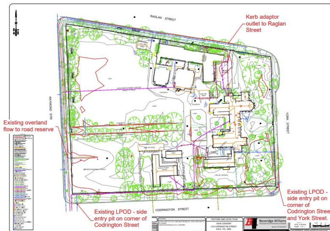
Figure 7 – Legal Point of Discharge
