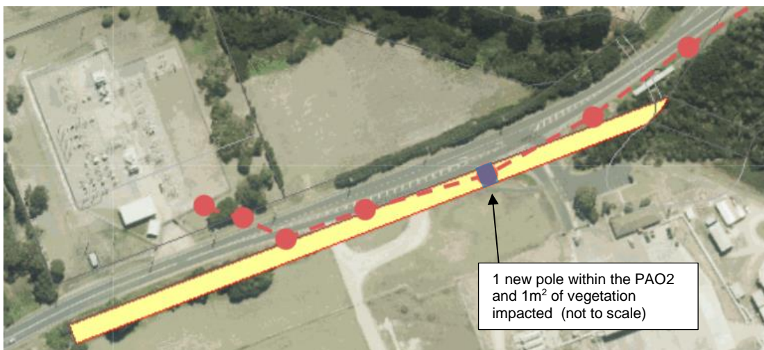
Figure 13. Works within the PAO2
