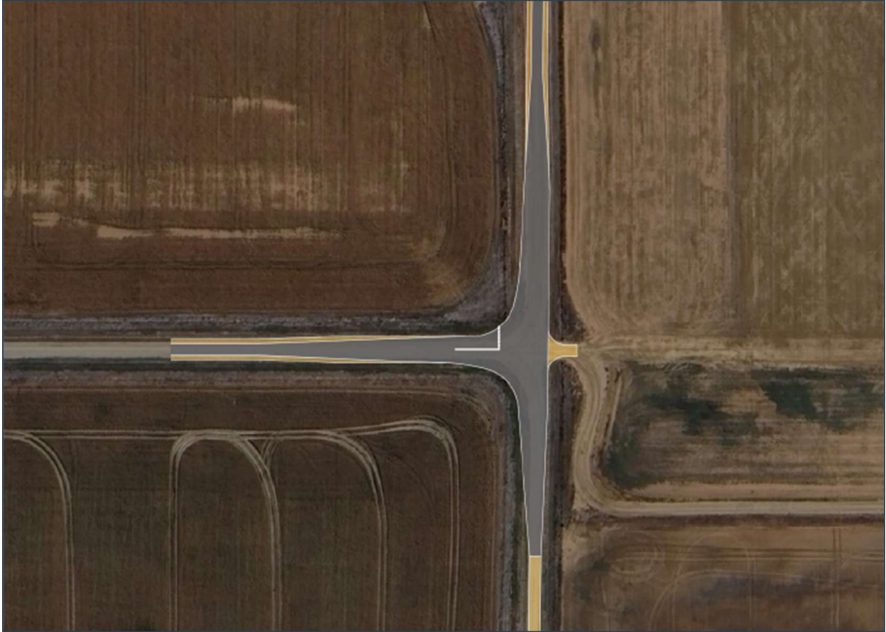
Figure 24: Baillieu Road / Chrystal Road Intersection Upgrade Concept (RMA Engineers 2025)
