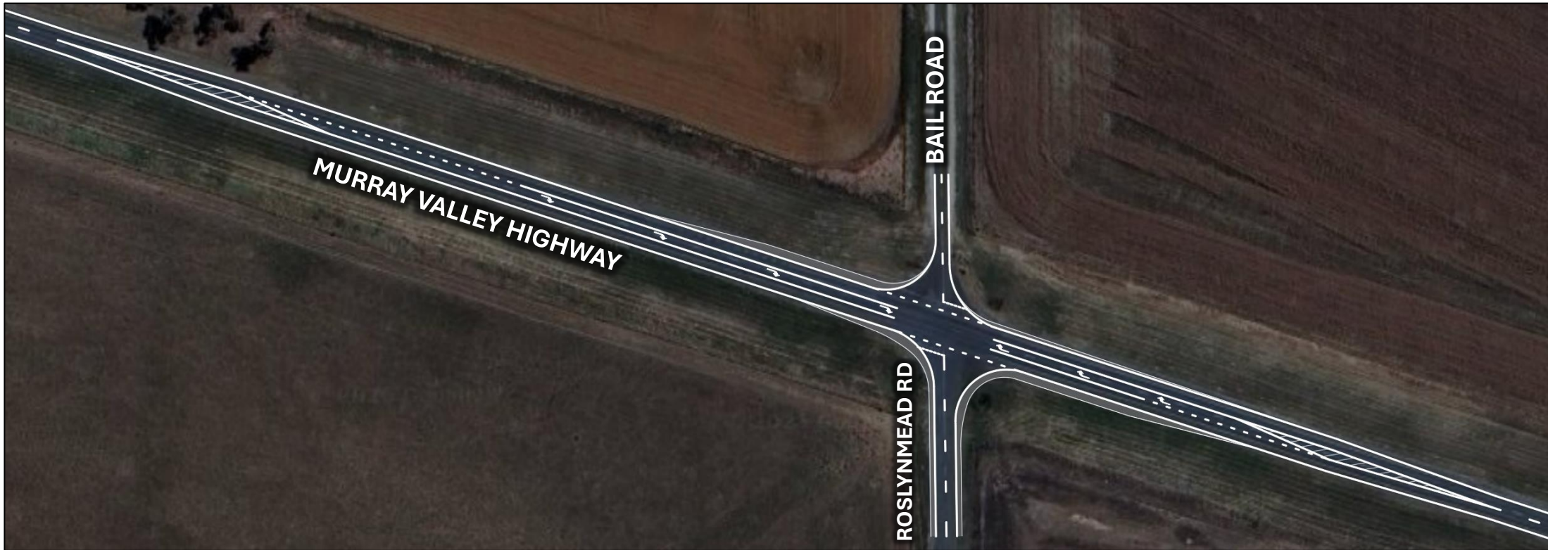
Murray Valley Highway / Roslynmead Road / Bail Road intersection upgrade concept sketch (CHR / CHR(S) / BAL layout)
