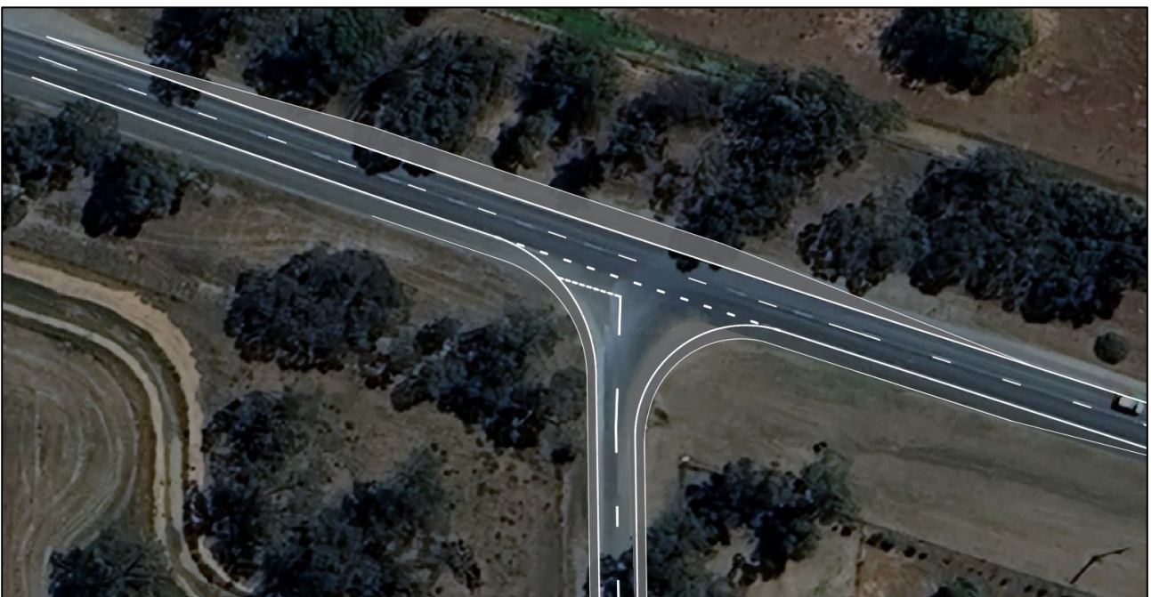
Figure 8-8: Murray Valley Highway / Davis Road intersection upgrade concept sketch
