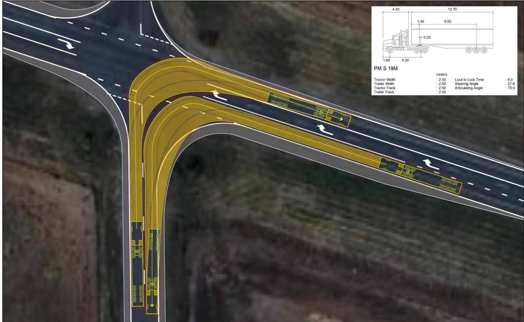
Murray Valley Highway / Roslynmead Road – 19m AV turn path – Left In / Right Out
