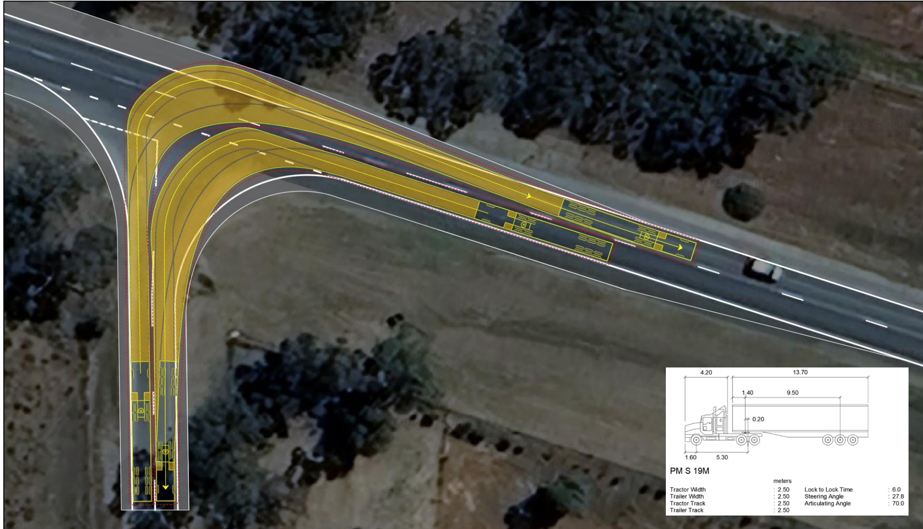
Murray Valley Highway / Davis Road – 19m AV turn path – Left In / Right Out
