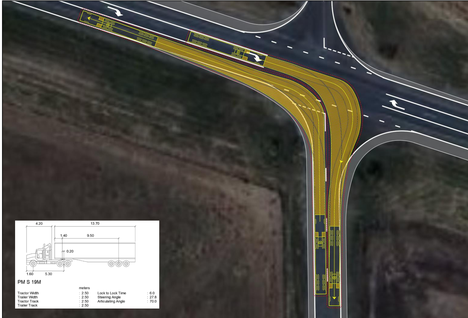
Murray Valley Highway / Roslynmead Road – 19m AV turn path – Right In / Left Out
