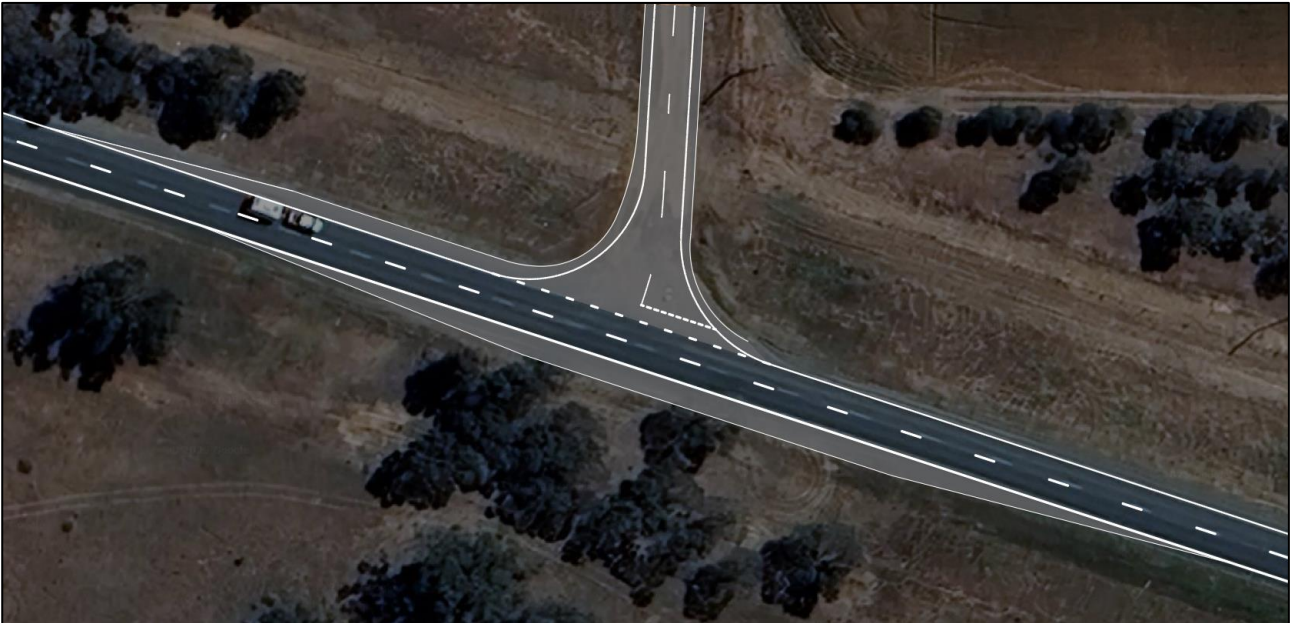
Figure 8-11: Murray Valley Highway / Heppell Road intersection upgrade concept sketch
