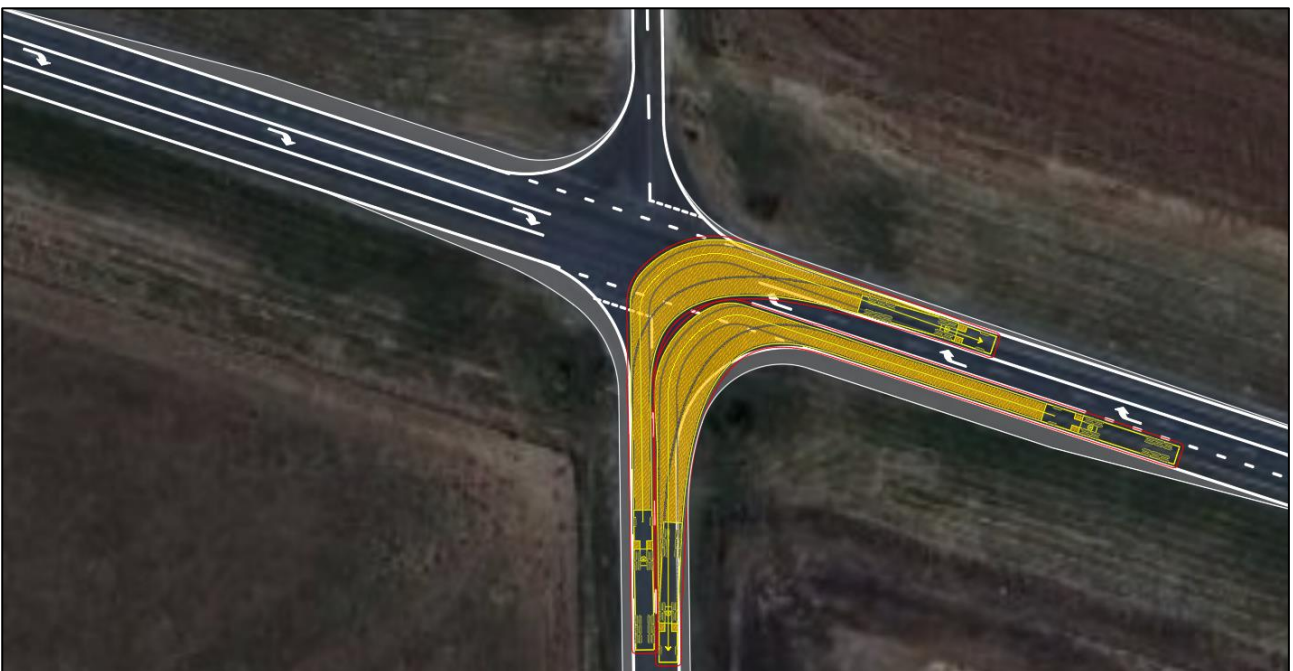
Figure 8-16: Murray Valley Highway / Roslynmead Road – 19m AV turn path – Left In / Right Out
