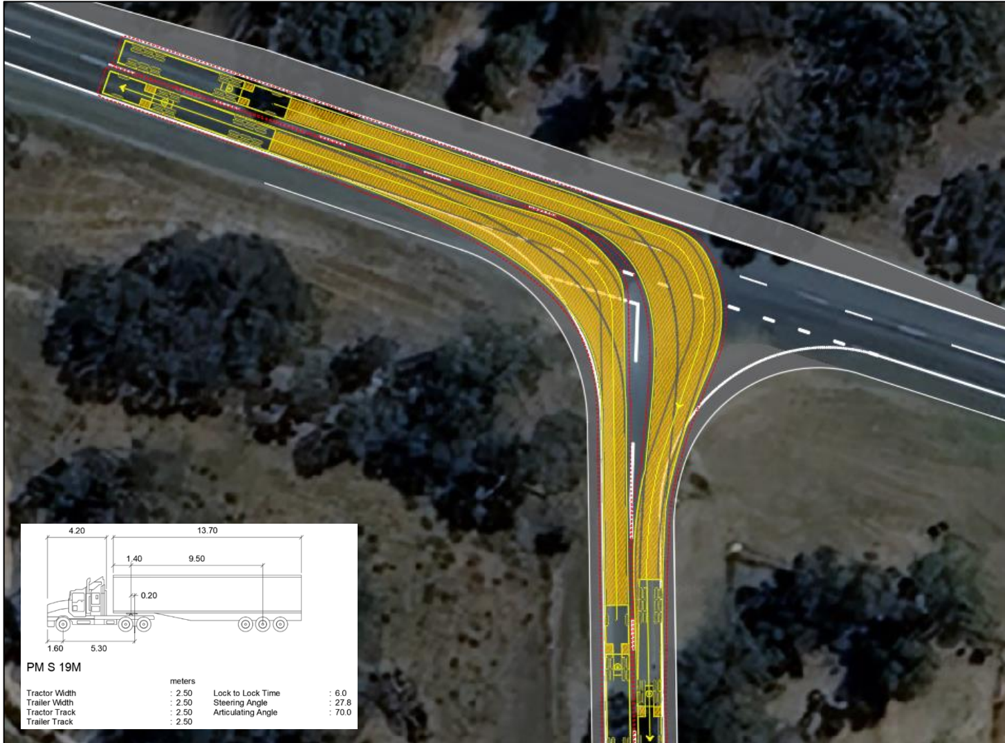
Murray Valley Highway / Davis Road – 19m AV turn path – Right In / Left Out
