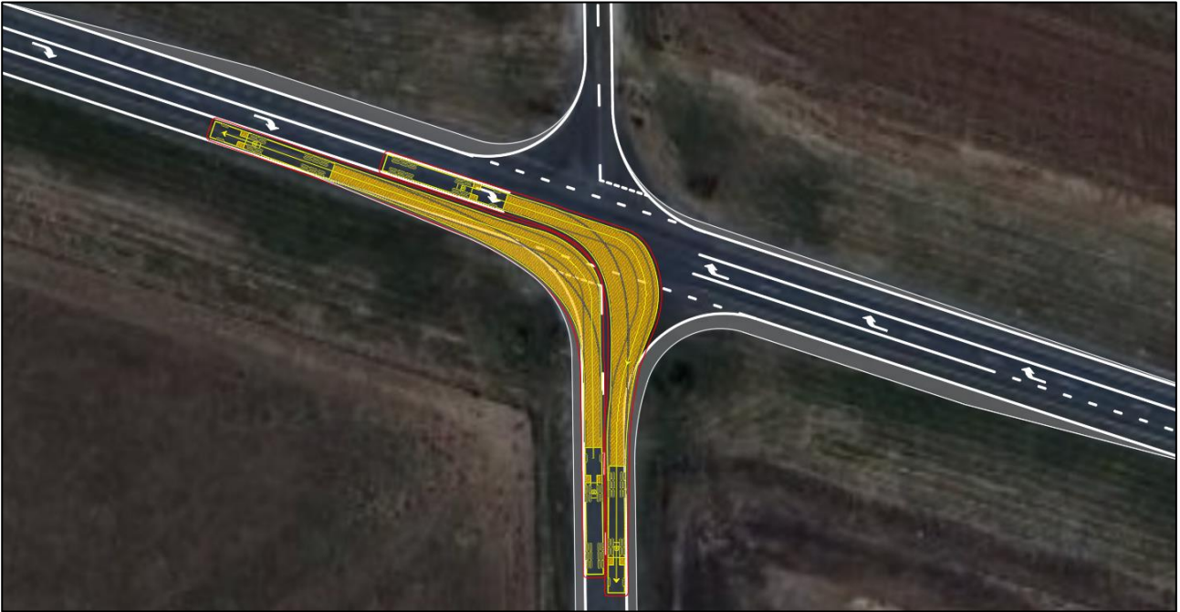
Figure 8-15: Murray Valley Highway / Roslynmead Road – 19m AV turn path – Right In / Left Out
