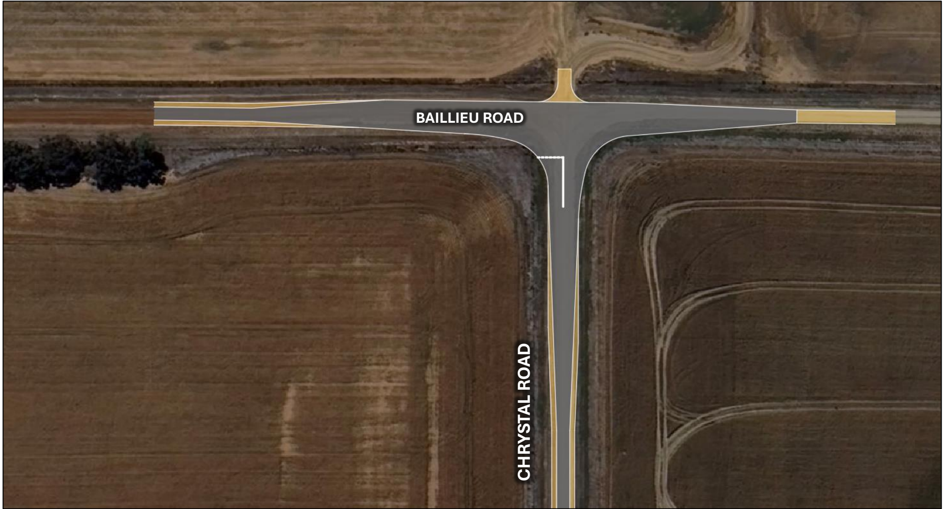
Baillieu Road / Chrystal Road intersection upgrade concept sketch (simple right and simple left layout)
