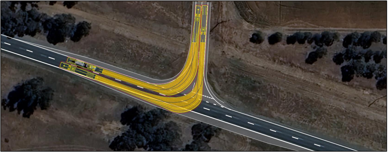
Figure 8-13: Murray Valley Highway / Heppell Road – 19m AV turn path – Left In / Right Out
