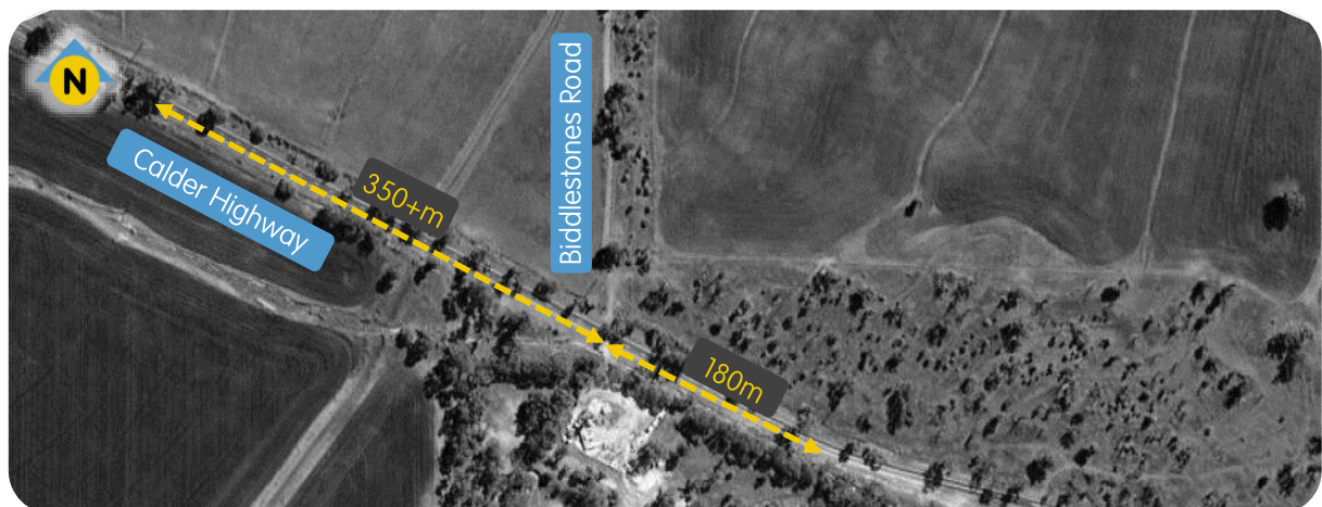
Figure 11 Sight Distance Assessment - Calder Highway & Biddlestones Road
