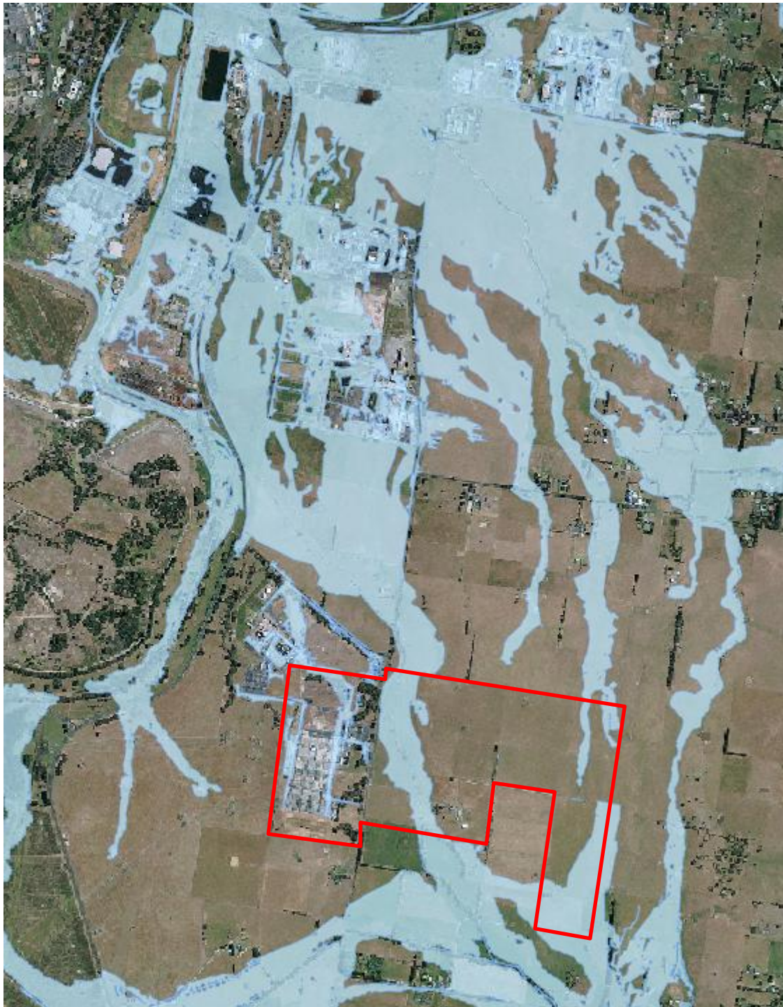
Figure 5-7: Areas of mapped 1% AEP flood extent (light blue) and site boundary (red outline) (Department of Transport and Planning, 2026)
