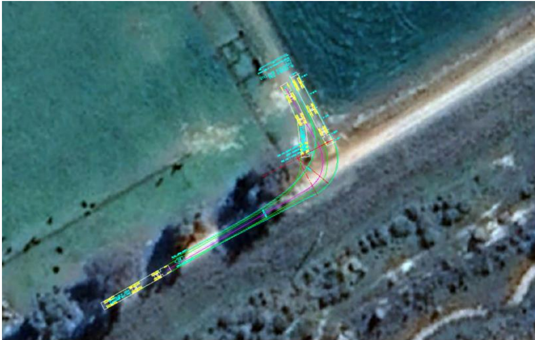
Figure 4-5 B-Double vehicle swept paths on existing geometry
