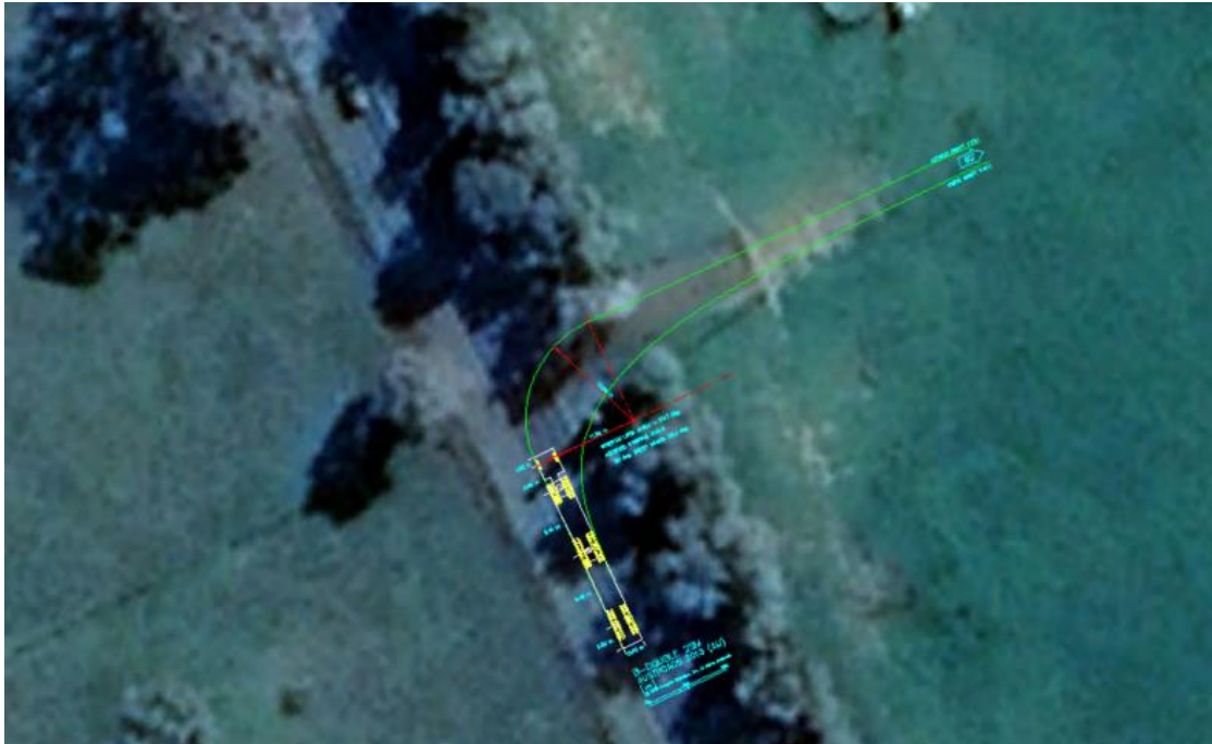
Figure 4-4 B-Double vehicle swept path on existing geometry of northernmost access located on Benalla-Yarrowonga Road
