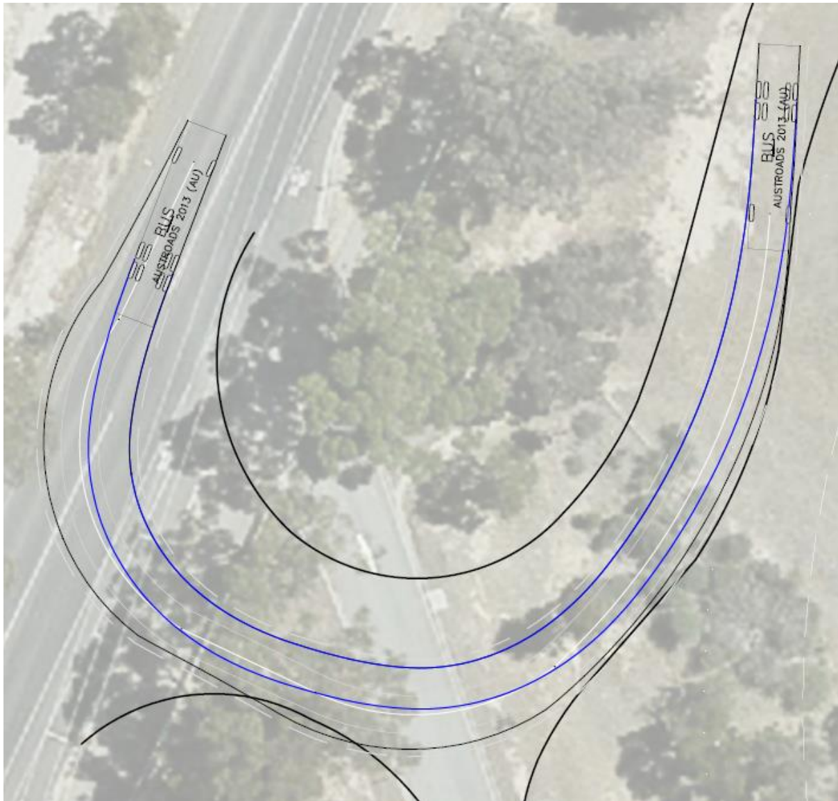
Figure 2-8 Turning movement – bus turning right into St Vincents Road from proposed carpark entrance
