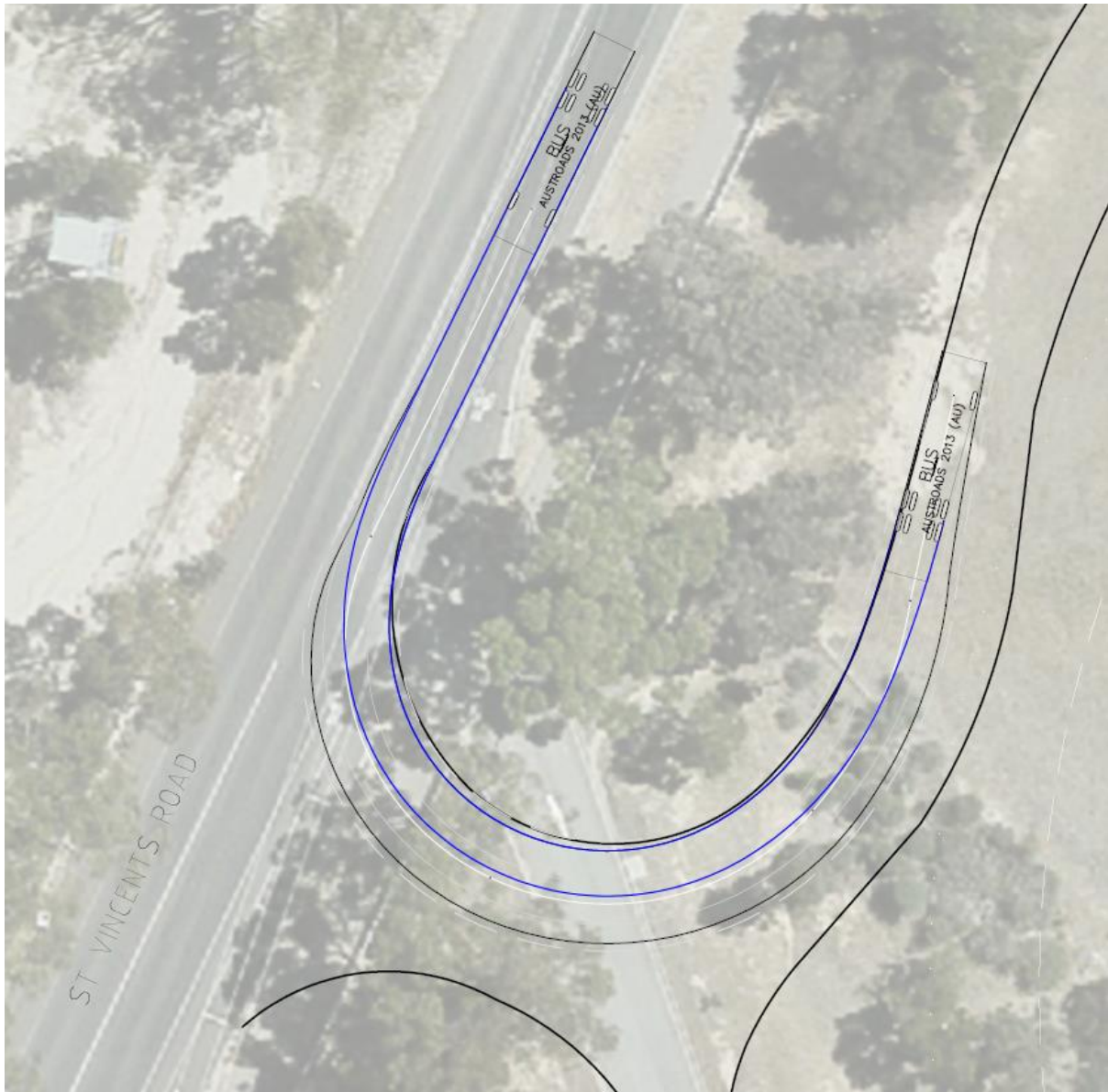
Figure 2-6 Turning movement – bus turning left from St Vincents Road into proposed carpark entrance
