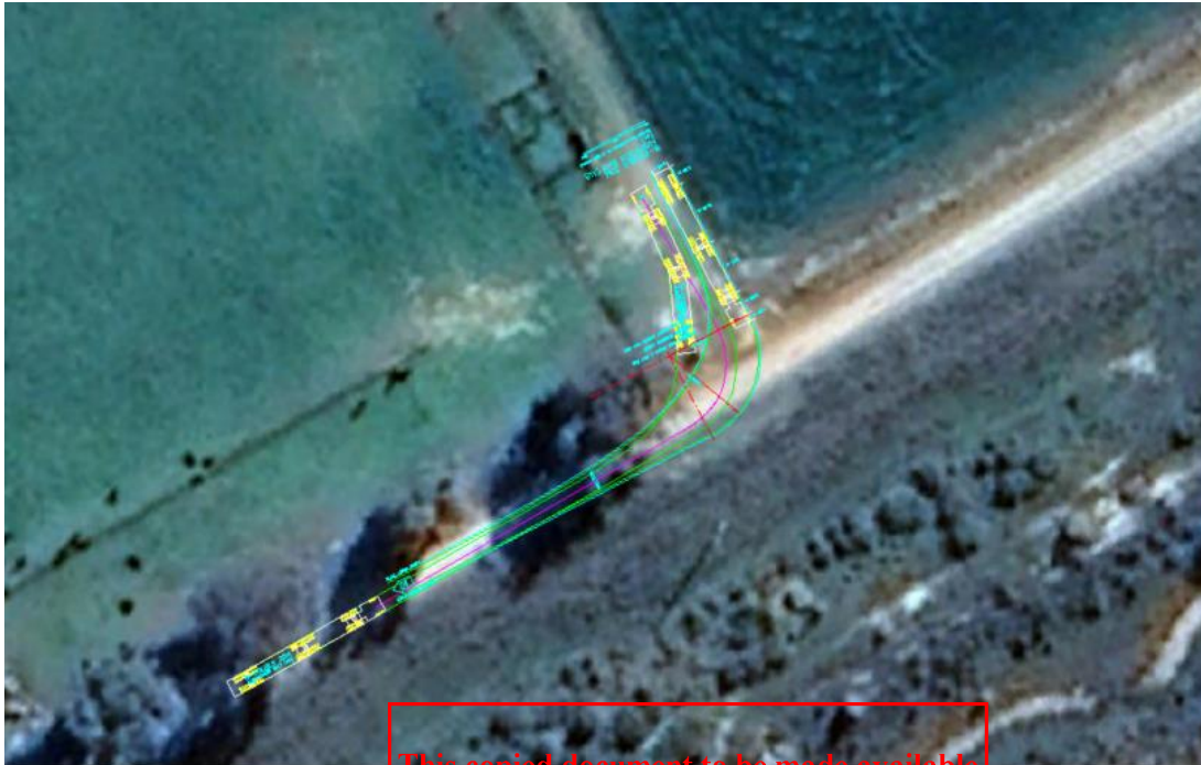
Figure 4-5 B-Double vehicle swept paths of existing geometry
