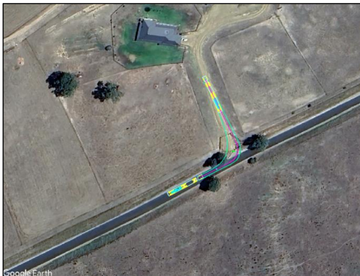
Figure 4-6 B-Double vehicle swept path on existing geometry of Lake Mokoan Road – Northeast Access Point
