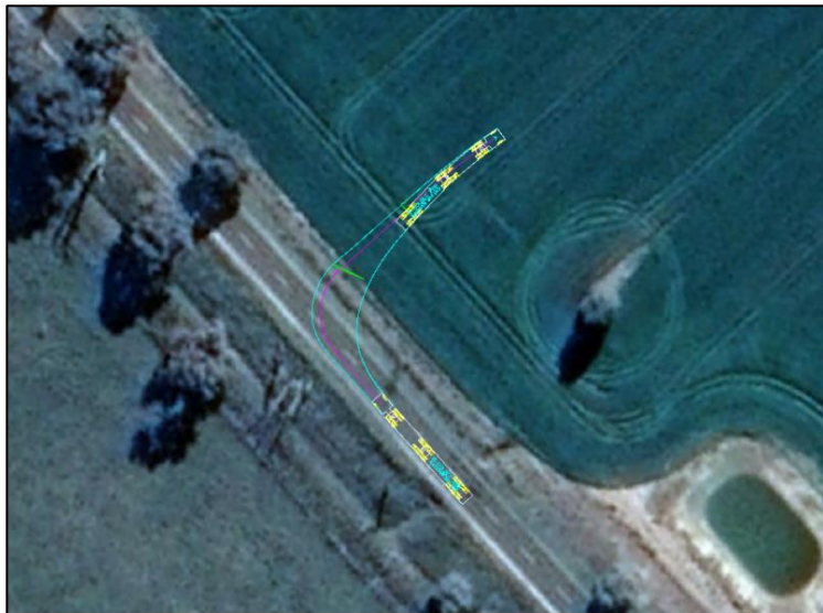
Figure 4-7 B-Double vehicle swept path analysis on existing geometry of Benalla-Yarrowonga Road – Northernmost Access Point
