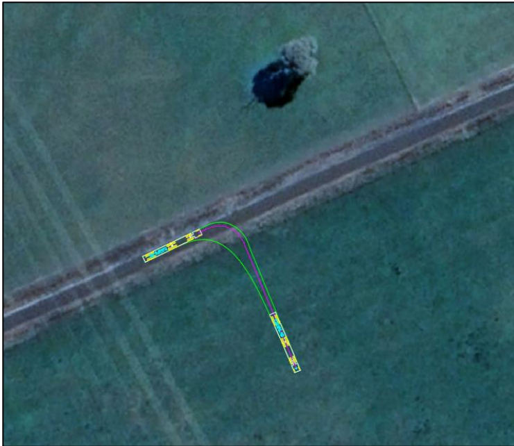
Figure 4-4 B-Double vehicle swept path on existing geometry of Lake Mokoan Road – Southwest Access Point
