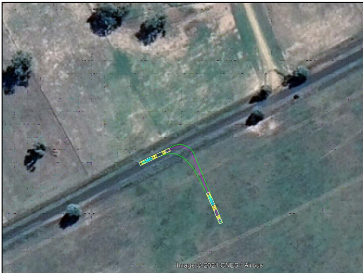
Figure 4-5 B-Double vehicle swept path on existing geometry of Lake Mokoan Road – Southeast Access Point
