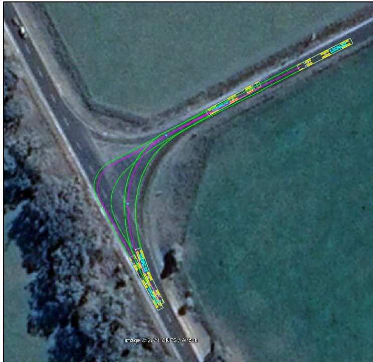
Figure 4-9 Two-way movement B-Double vehicle swept path on existing geometry of Benalla-Yarrowonga Road and Lake Mokoan Road intersection
