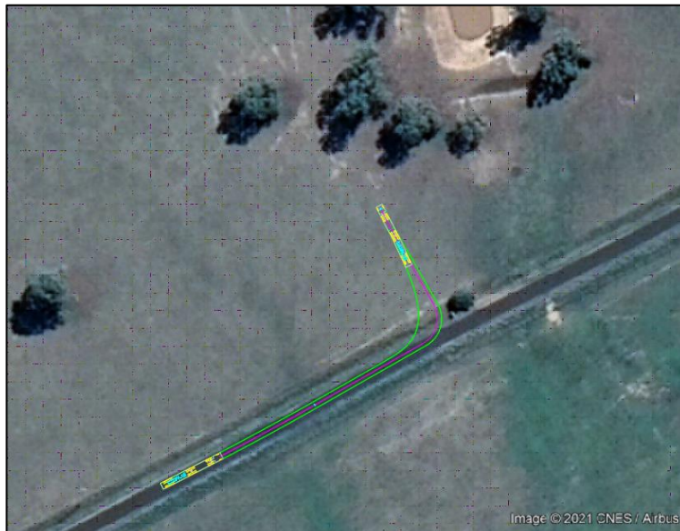
Figure 4-3 B- Double vehicle swept path on existing geometry of Lake Mokoan Road – Northwesternmost Access Point
