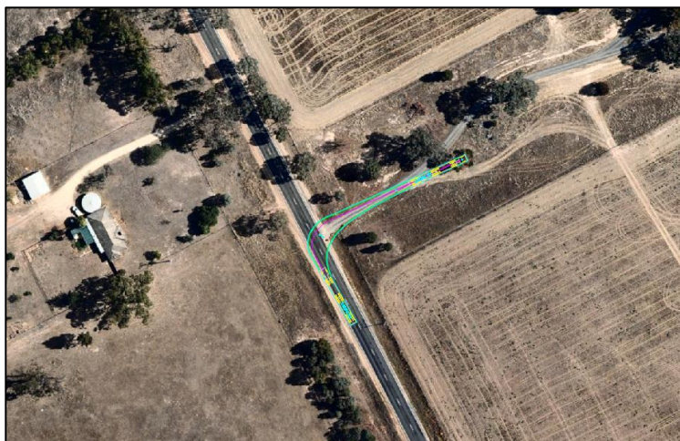
Figure 4-8 B-Double vehicle swept path analysis on existing geometry of Benalla-Yarrowonga Road – Southernmost Access Point
