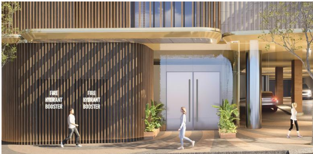
Image 7 example of secure external booster and adjacent plant – SOM Architecture
