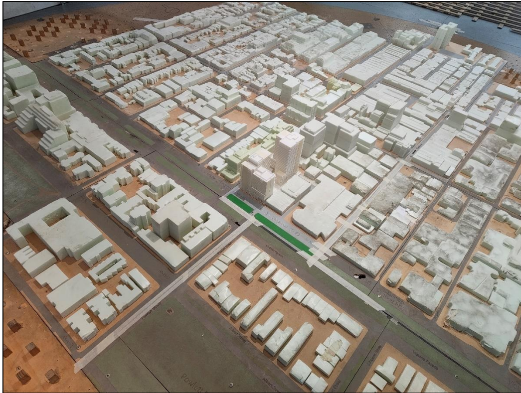
Figure 2b - View from the southeast of the 1/400 scale model of the proposed 79-81 Victoria Parade development in the wind tunnel.
