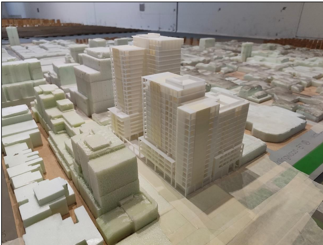
Figure 2a - View from the southwest of the 1/400 scale model of the proposed 79-81 Victoria Parade development in the wind tunnel.
