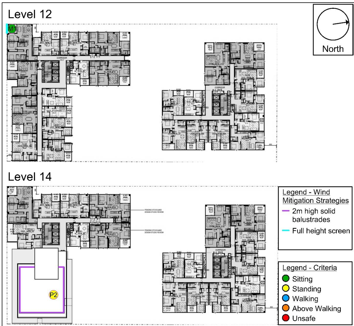
Figure 7a - Summary of wind criteria satisfied on Level 12 and 14 of the 79-81 Victoria Parade development for the Proposed Configuration with wind mitigation strategies.
