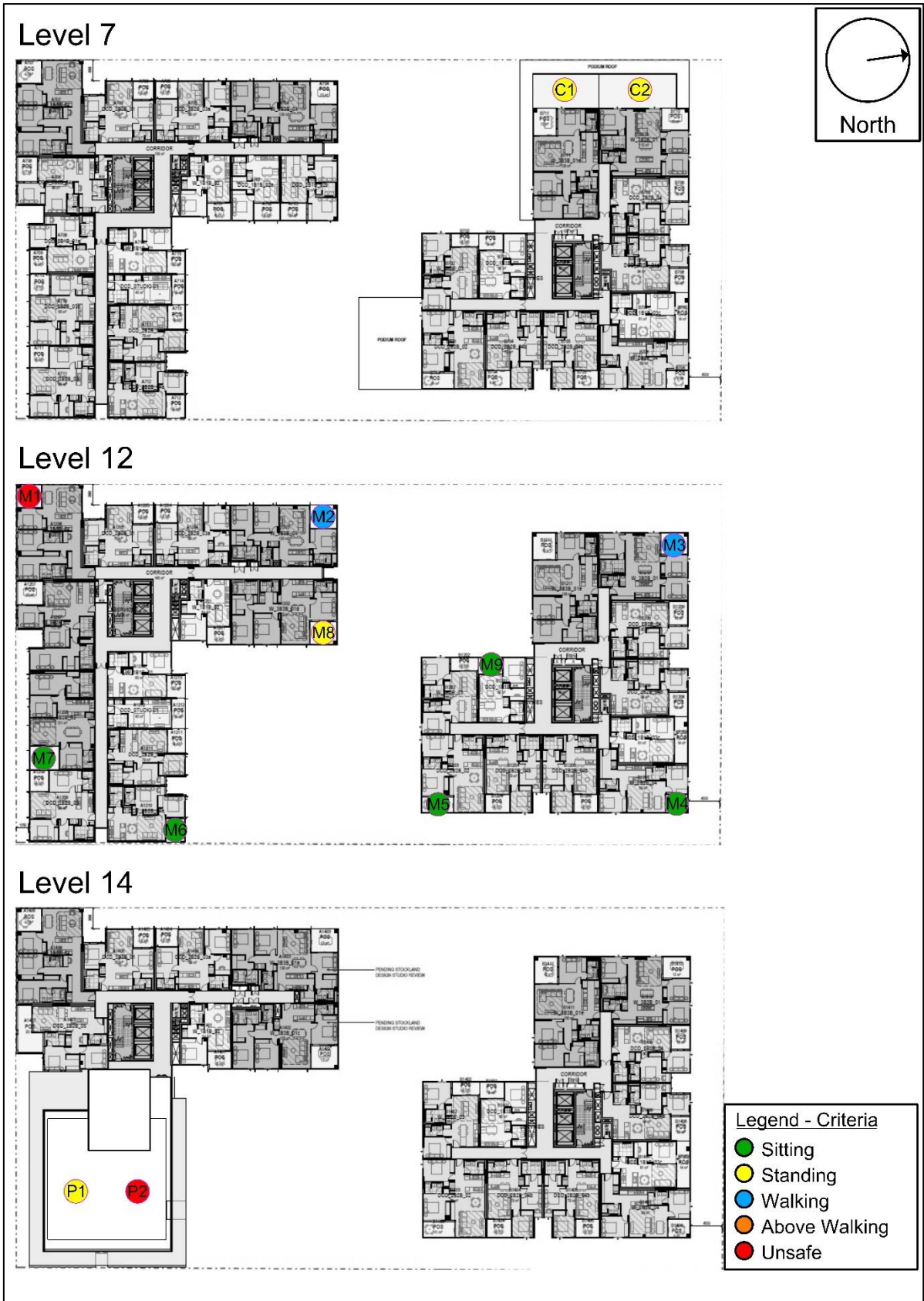
Figure 6c - Summary of wind criteria satisfied on the Level 7, 12 and 14 terraces of the 79-81 Victoria Parade development for the Proposed Configuration.
